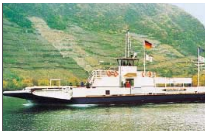
Double-ended ferry (0.75 m draught), 2 x SPJ 57 (178 kW each) Shipyard: Schmitt Stahlbau GmbH, Germany Owner: Fährbetrieb Michael Schnaas, Germany
