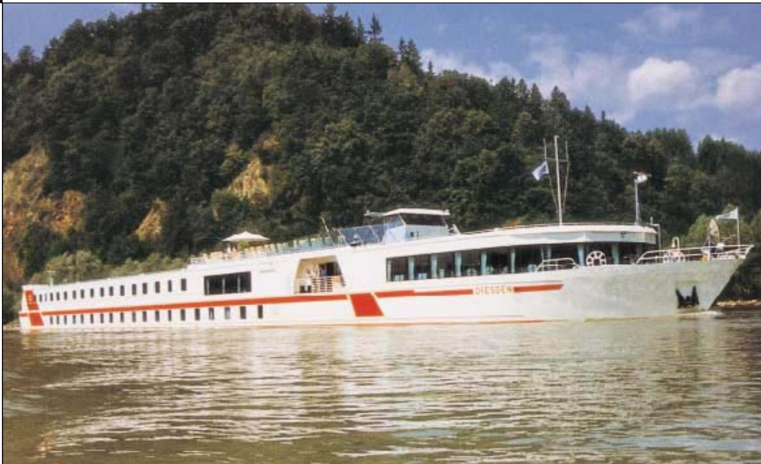
River cruise vessel (0.90 m draught), 3 x SPJ 82 (340 kW each) stern installation, 1 x SPJ 57 (190 kW) bow installation Shipyard: DWE Deggendorfer Werft & Eisenbau GmbH, Germany Owner: Peter Deilmann Reederei GmbH & Co., Germany
