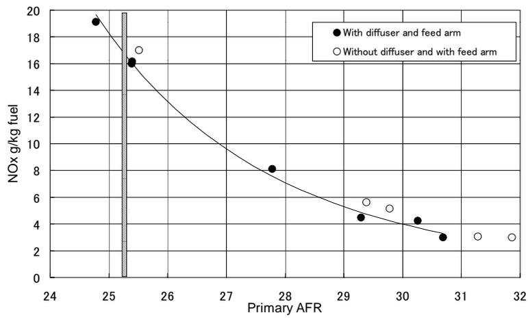
Figure 9 NOx emission comparison between the units with & without diffuser
