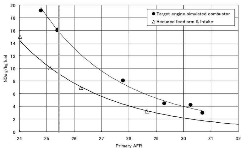
Figure 10 NOx emission comparison between the units with & without feed arm
