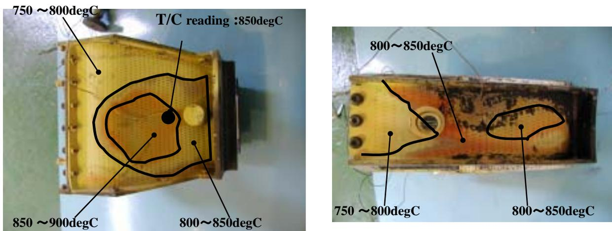
Figure 13 Angled effusion liner thermal paint results
