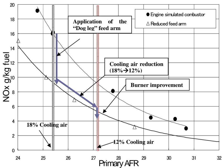
Figure 12 Further NOx reduction plan
