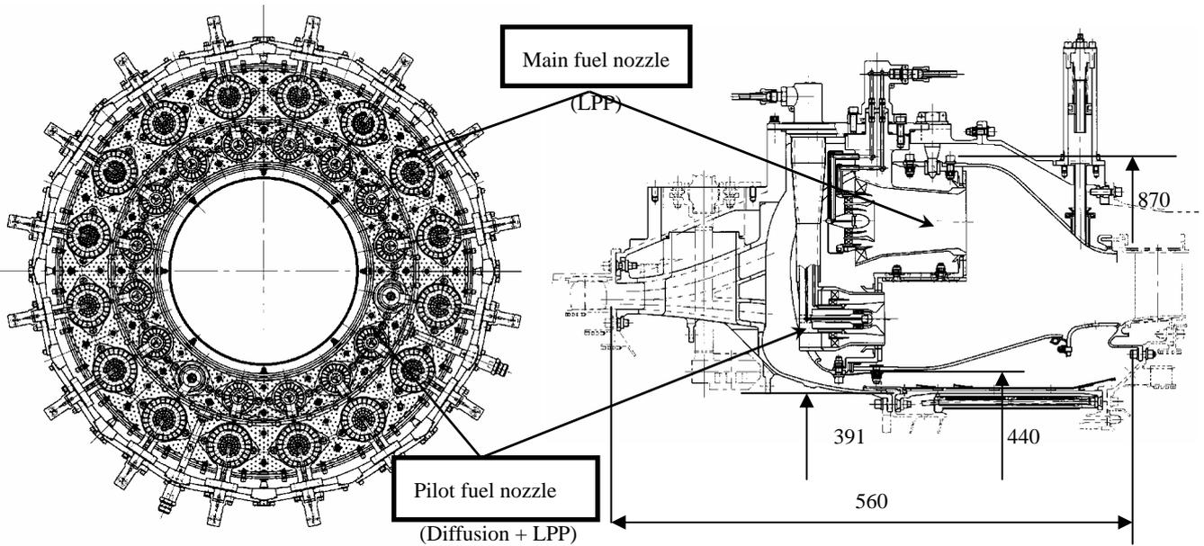
Figure 2 ESPR axially staged combustor
