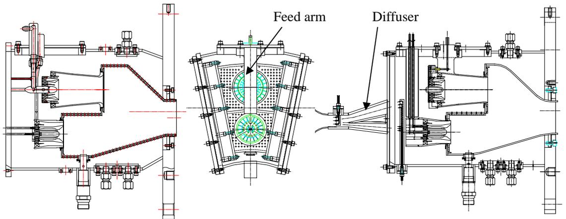
Figure 6 Single sector combustor test unit
