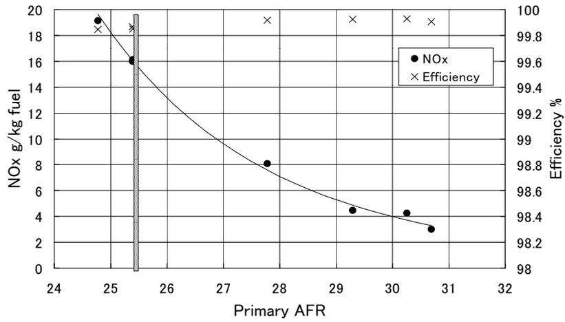
Figure 8 NOx emission and combustion efficiency (engine simulated combustor)
