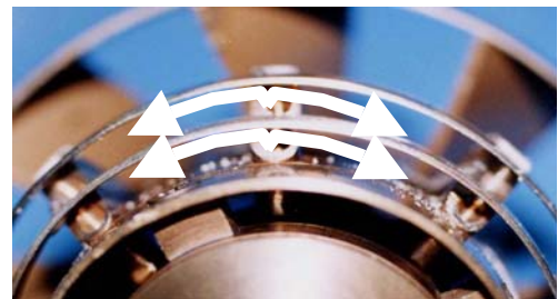
Fig. 17 Picture of the fuel supply unit with the main plates from the upstream view (J)
