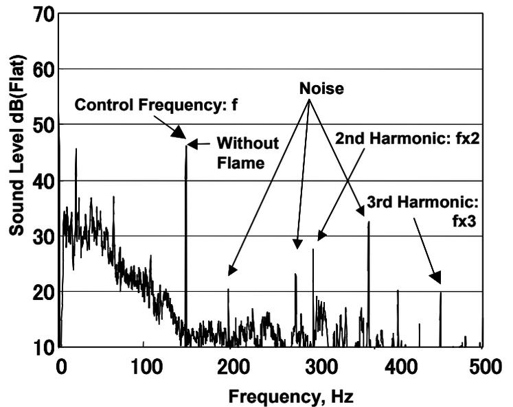
Fig. 8(a) Spectrum of Sound Emitted by Oscillating Fuel Flow
