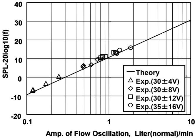
Fig. 7 Comparison between Experiment and Theory for Flow Rate Oscillation
