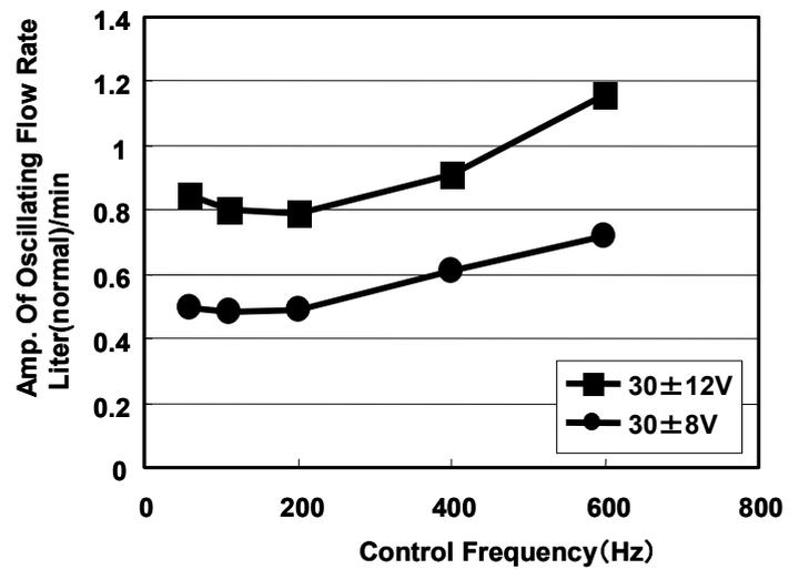
Fig.6 Amplitude of Flow Rate Oscillation
