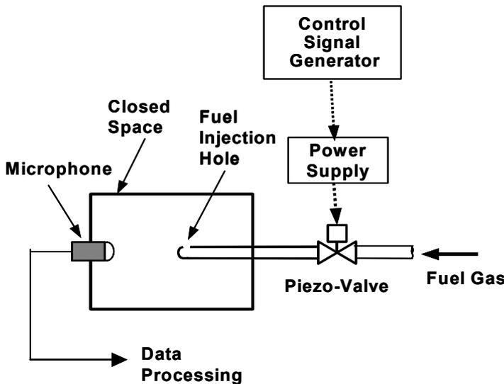
Fig.5 Experimental Scheme of Flow Rate Measurement
