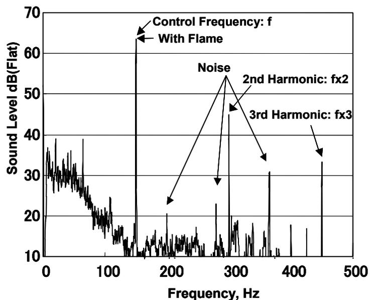
Fig. 8(b) Spectrum of Sound Emitted by Oscillating Flame
