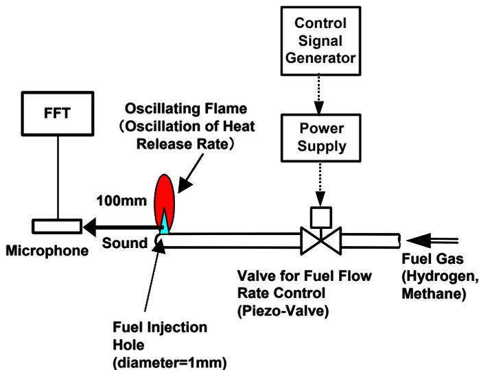
Fig.2 Experimental Scheme of Sound Measurement
