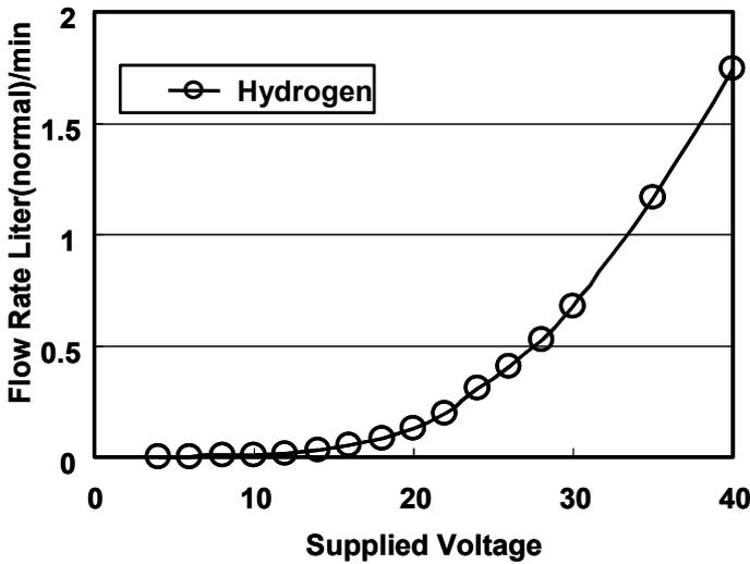
Fig.4 Relation between Static Flow Rate and Input Voltage
