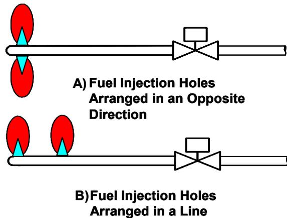
Fig. 13 Fuel Injection Holes Arrangement
