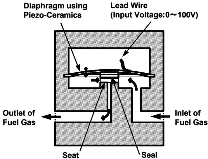
Fig.1 Structure of Piezo-Valve
