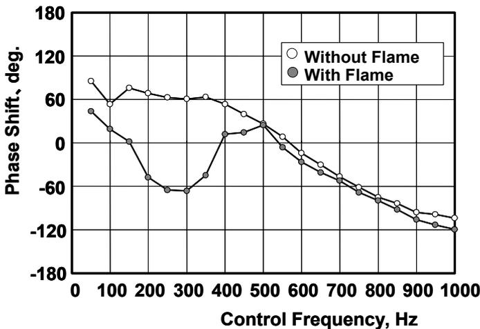
Fig. 12 Phase Shift from Input Control Signal
