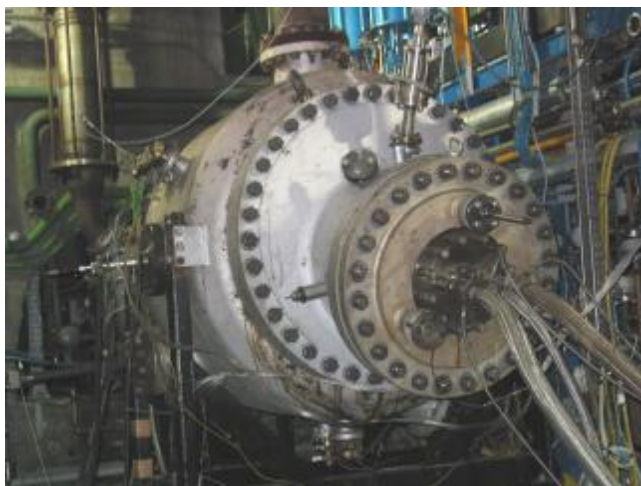
Fig. 9 The combustor at the Full pressure test rig of Sesta
