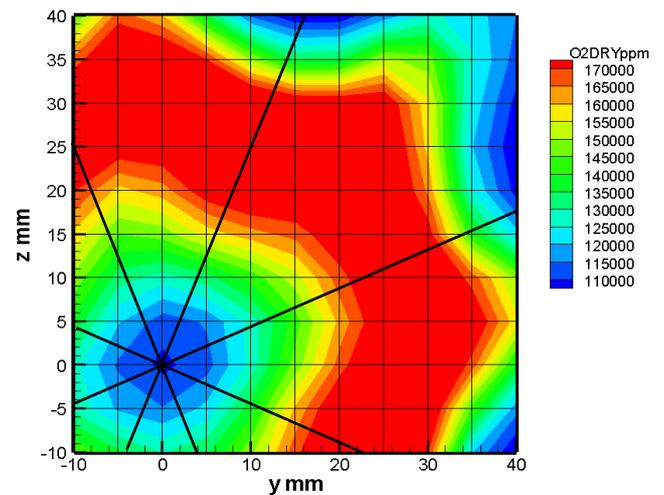
Fig. 6 O<sub>2</sub> concentration distribution at x=-200 (Uc=15, Ta=700, ERc=0.50, PP=3.0)
