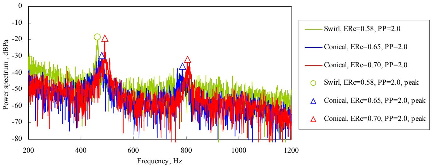
Fig. 14 Power spectrums of pressure in combustion chamber
