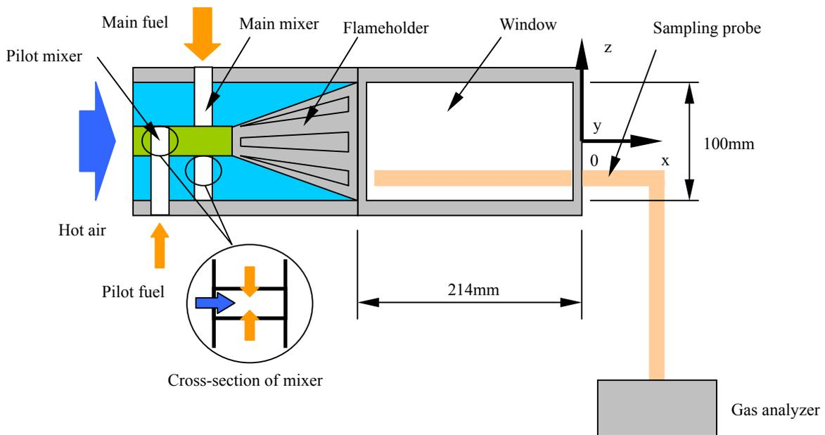
Fig. 4 Schematic of test rig
