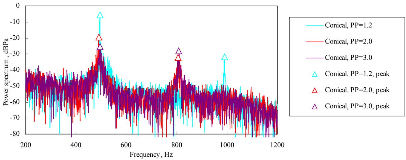
Fig. 15 Influence of PP on power spectrums of pressure
