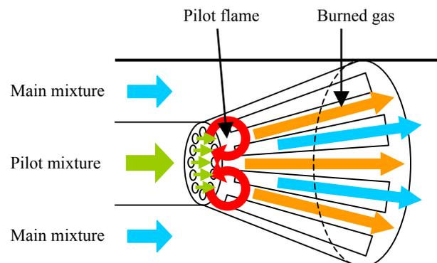
Fig. 1 Concept of conical flameholder
