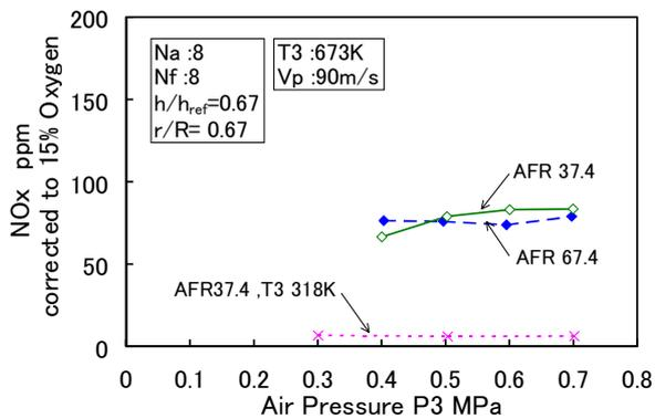
Fig 3 Relation between inlet air pressure and NOx emission (Multi-port version)
