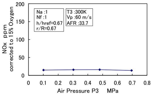
Fig 2 Relation between inlet air pressure and NOx emission (Single-port version)
