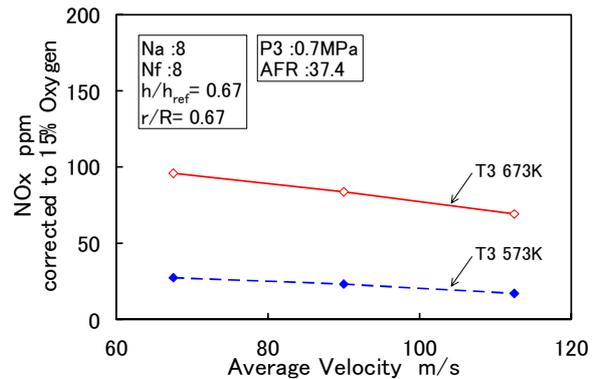
Fig 5 Relation between air inlet velocity and NOx emission
