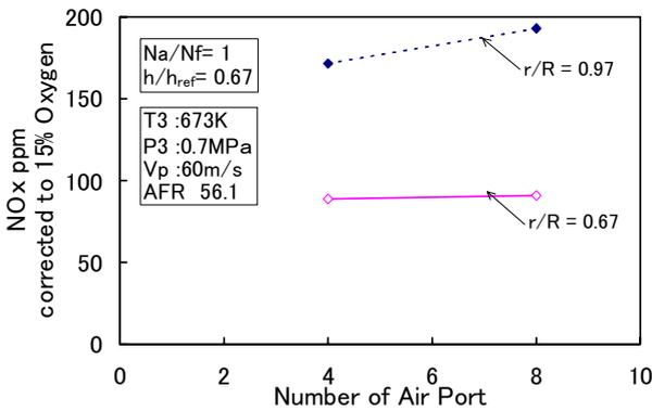
Fig.7 Relation between Number of Inlet-Air Ports and NOx emission
