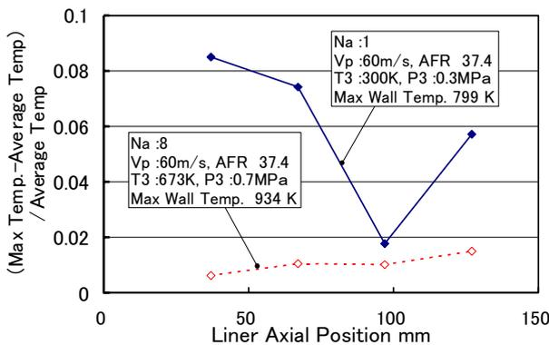
Fig.8 Comparison of wall temperature uniformity for single and multi port burner
