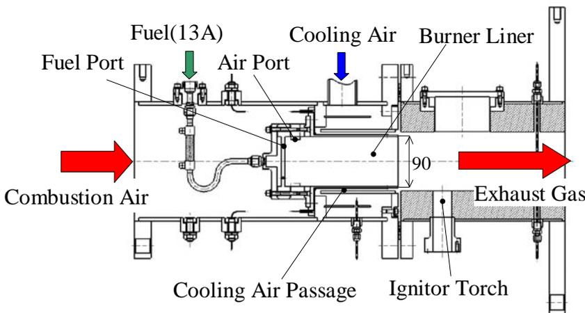
(b) Burner test rig
