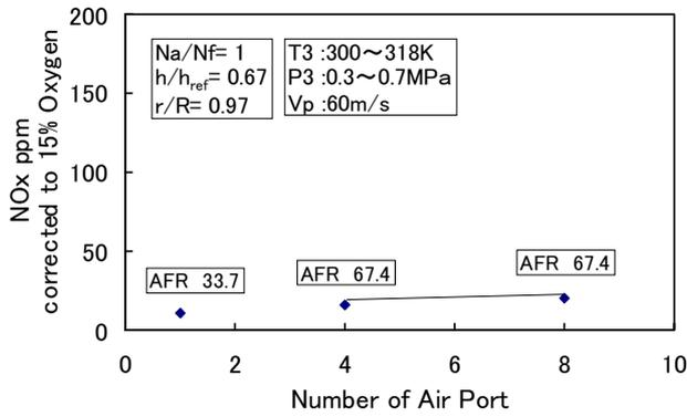
Fig.6 Relation between number of inlet-air ports and NOx emission
