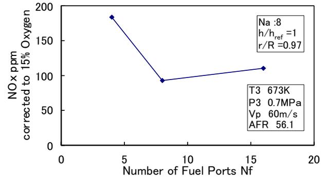
Fig.9 Relation between number of fuel ports and NOx emission
