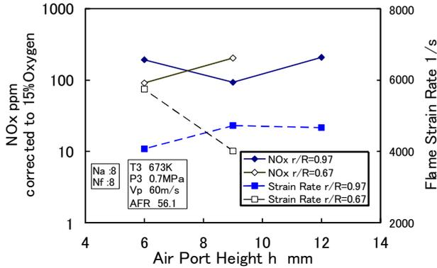
Fig 10 Effect of air port height on NOx emission for two different fuel injection positions and its relation to flame strain rate
