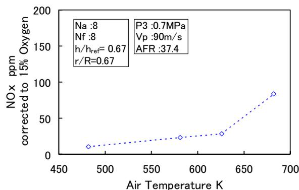
Fig 4 Relation between inlet air temperature and NOx emission (Multi-port version)
