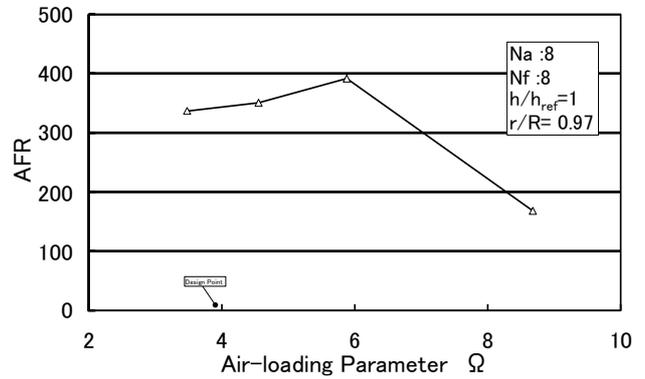
Fig 12 Blow off limit of spiral flame burner
