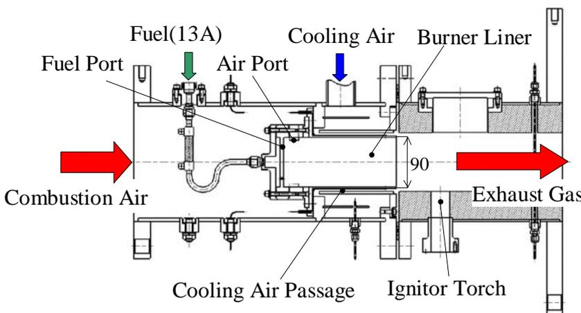
(b) Burner test rig
