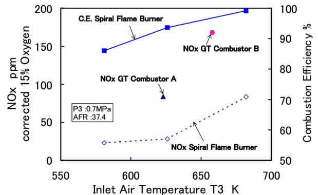
Fig 13 Comparison of NOx emission for spiral flame combustor and conventional non-premixed combustors
