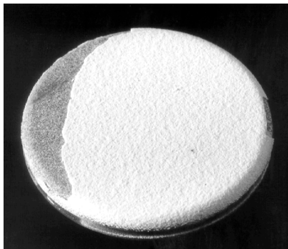
Fig. 8 \text{La}_2\text{Zr}_2\text{O}_7 single layer TBC after 960 cycles with a mean bond coat and surface temperatures of 1010°C and 1241°C, respectively.
