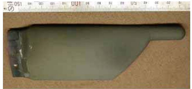
Fig. 14 Casting mold made by plasma spraying
