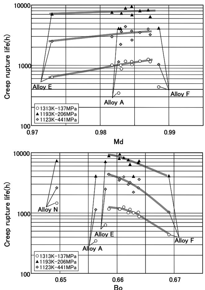
**Fig.3** Effects of Md and Bo on the creep rupture life.
