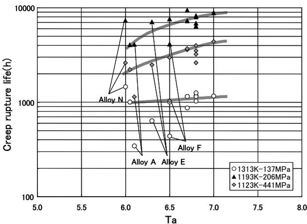
Fig.4 Effects of alloy elements on the creep rupture life.
