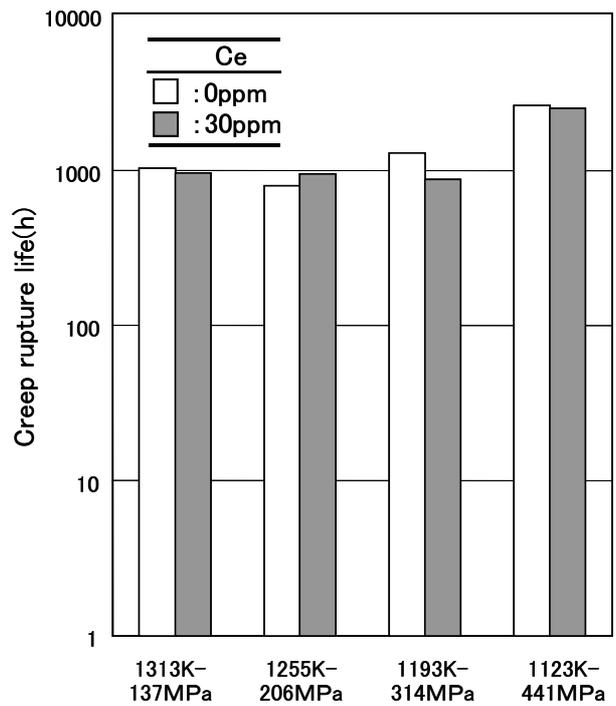
Fig.10 Creep rupture lives of the alloy G with Ce addition and Ce free alloy G.
