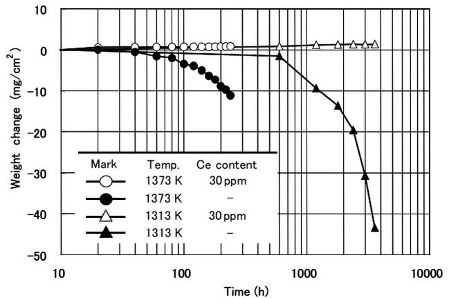
Fig.8 Result of oxidation test.
