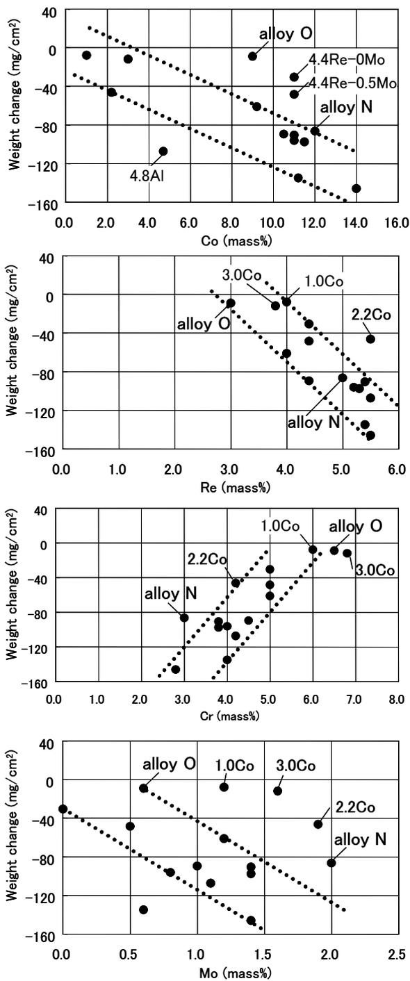
Fig.6 Effects of alloy elements on the weight change in oxidation tests.(1313K-3000h)
