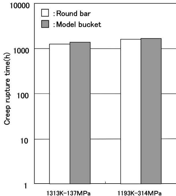
Fig.14 Creep rupture strength of the specimen that was cut down from the single crystal model bucket and round bar specimen.
