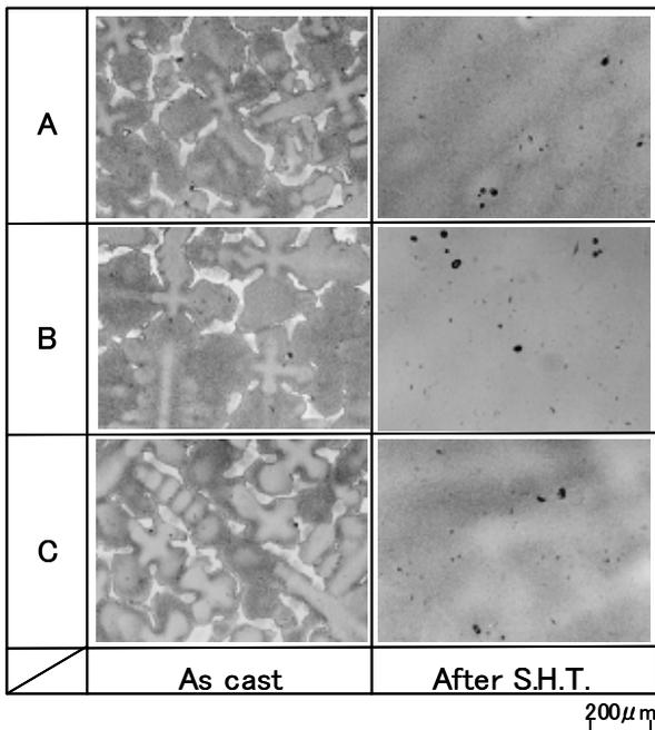
Fig.12 Cross-sectional microstructures of the model bucket. (S.H.T:Solution Heat Treatment)
