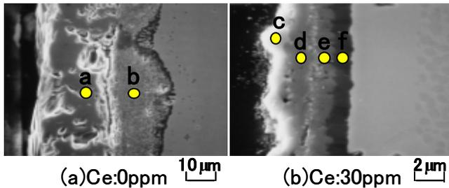
Fig.9 SEM micrographs of surface scale.
