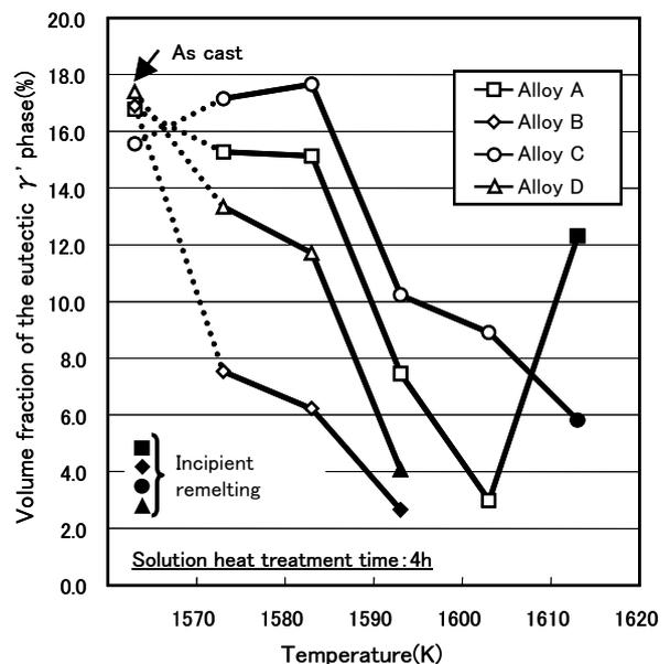
Fig.2 Effect of solution heat treatment on volume fraction of the eutectic  $\gamma'$  phase.
