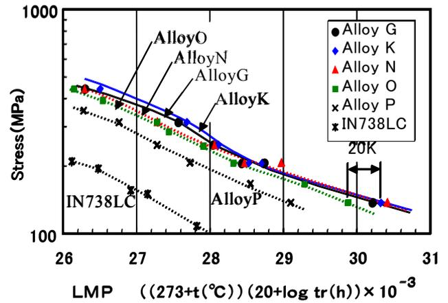
Fig.5 Creep rupture strength of alloy studied.
