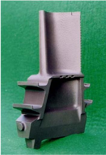
Fig.11 Overview of trially casted model bucket.(length: 170mm)
