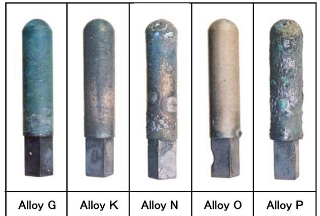
Fig.7 Overview of test specimens after burner rig tests and weight changes for the tests.
