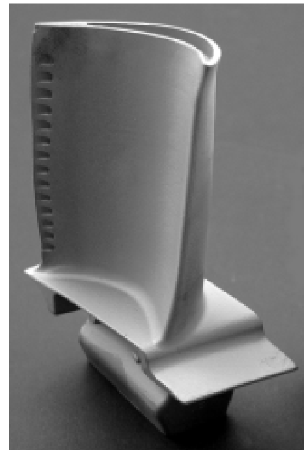
Fig. 11 Typical HPT blade of TMS-138 alloy.
