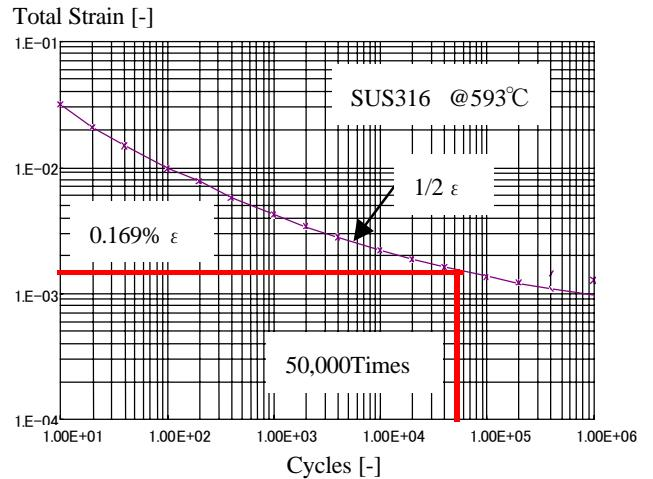
**Fig.12 Evaluation of Low Cycle Fatigue at the Hot Air Header Tank (Collector)**
