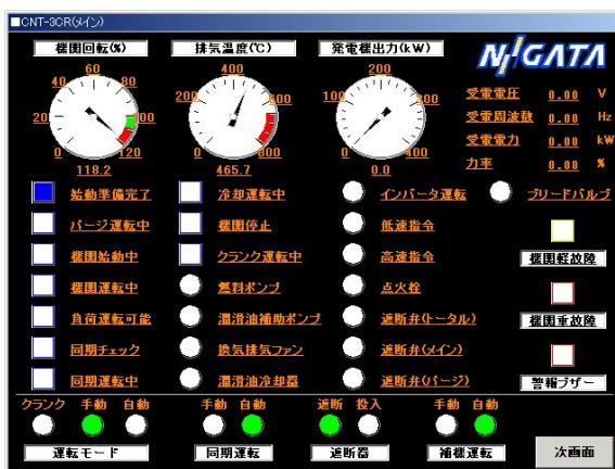
**Fig.15 An Example of LCD Man-Machine Interface Panel**
