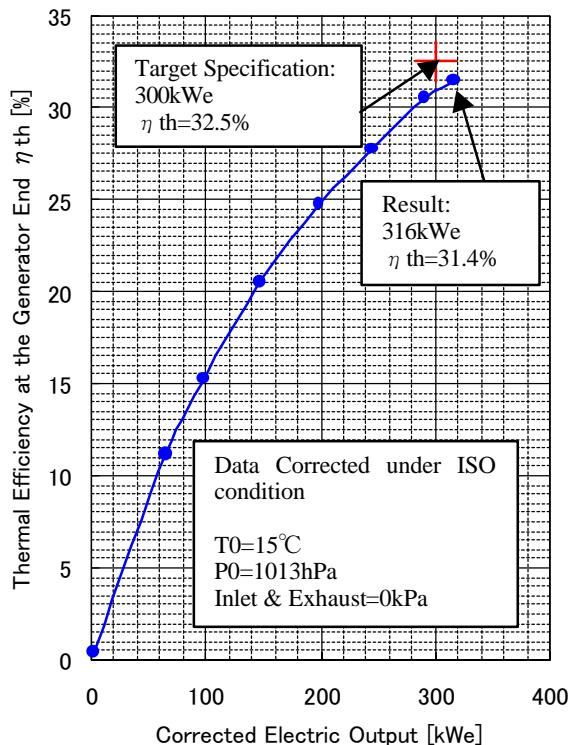
**Fig.19. Thermal Efficiency of prototype RGT3R**
