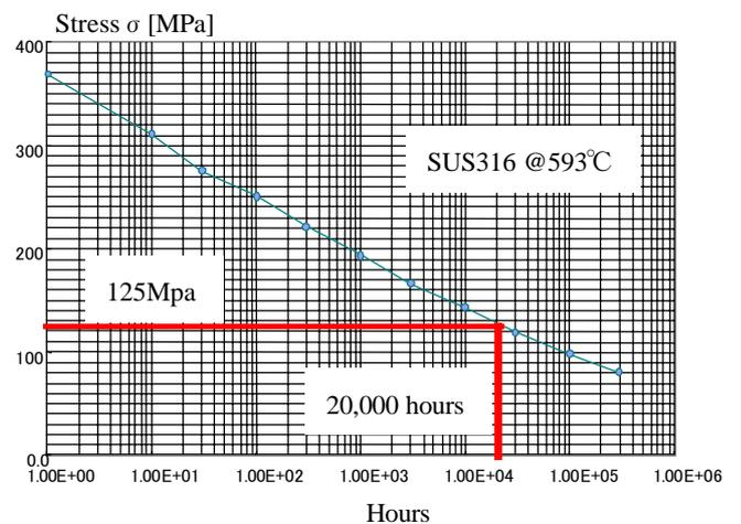
**Fig.13 Evaluation of Creep Rupture at the Hot Air Header Tank (Collector)**
