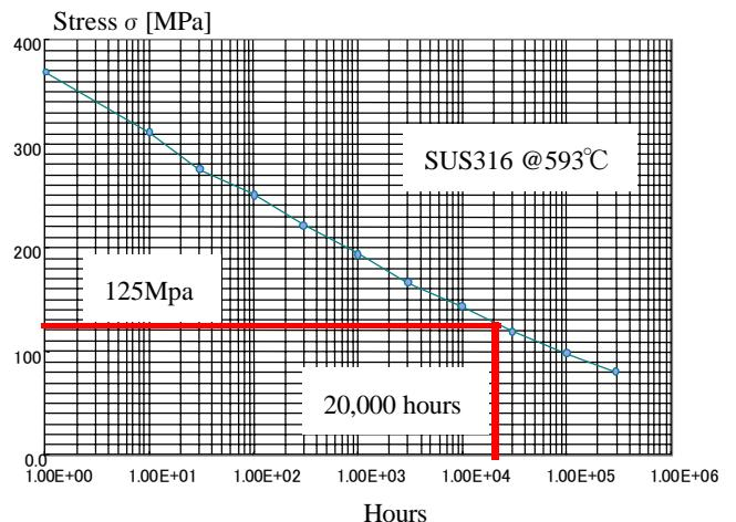
**Fig.13 Evaluation of Creep Rapture at the Hot Air Header Tank (Collector)**
