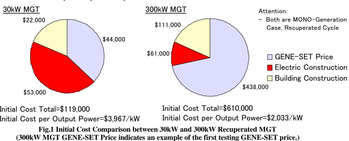
Fig.1 Initial Cost Comparison between 30kW and 300kW Recuperated MGT
