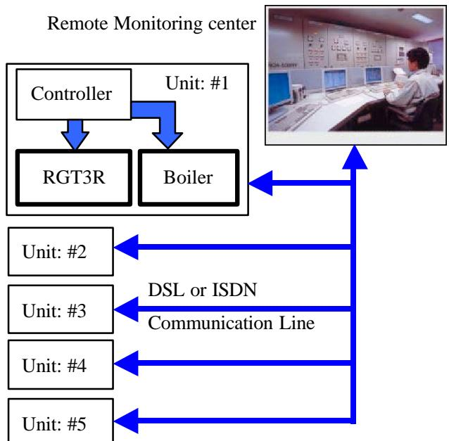
**Fig.16 A Schematic of Remote Monitoring System**
