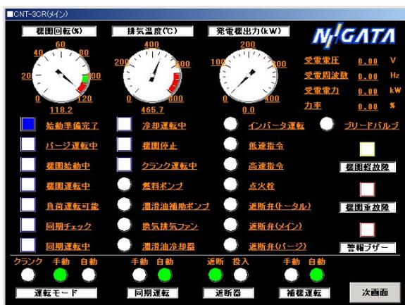
Fig.15 An Example of LCD Man-Machine Interface Panel
