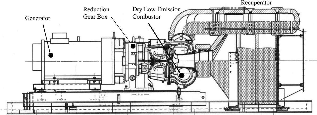
**Fig. 2 Cross Sectional View of RGT3R**
