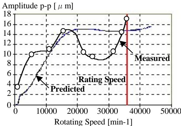
**Fig.7 Comparison between Unbalance Response analysis Prediction and Test Data at the Rotor Output Coupling end.**
