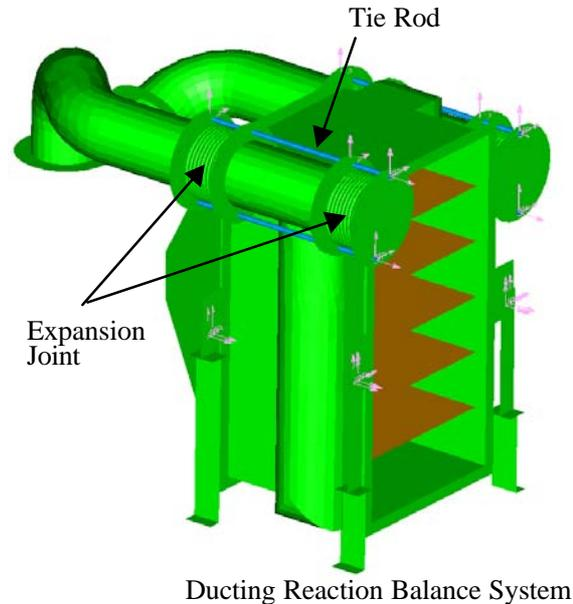
**Fig.10 Schematics Recuperator Support (on the left) and Ducting Reaction Balance System (on the right).**
