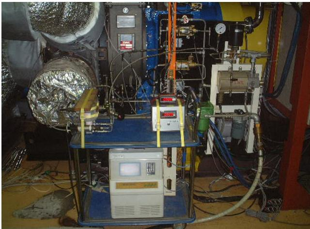
**Fig.17 Prototype RGT3R equipped with Dry Low Emission Combustor**
