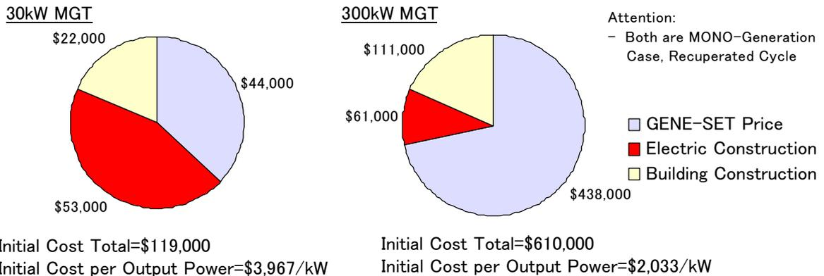
Fig.1 Initial Cost Comparison between 30kW and 300kW Recuperated MGT (300kW MGT GENE-SET Price indicates an example of the first testing GENE-SET price.)
