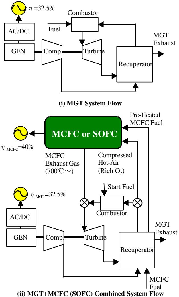
Fig.20 A Schematic of MCFC (SOFC) and Recuperated MGT Combined System
