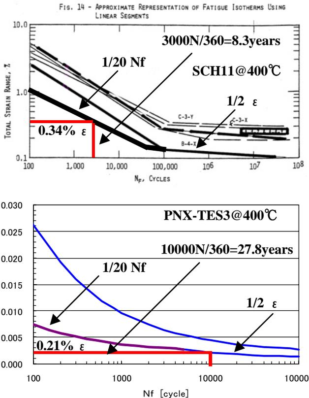
Fig.9 Low Cycle Fatigue Life of the RGT3R Turbine Casing Evaluated in accordance with ASME N-47 code (Upper: SCH11 / Lower: PNX-TES3 @400°C)
