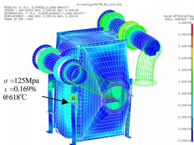
**Fig.11 FEM analysis of the final Recuperator and Ducting configuration.**
