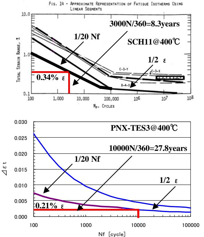
**Fig.9 Low Cycle Fatigue Life of the RGT3R Turbine Casing Evaluated in accordance with ASME N-47 code
