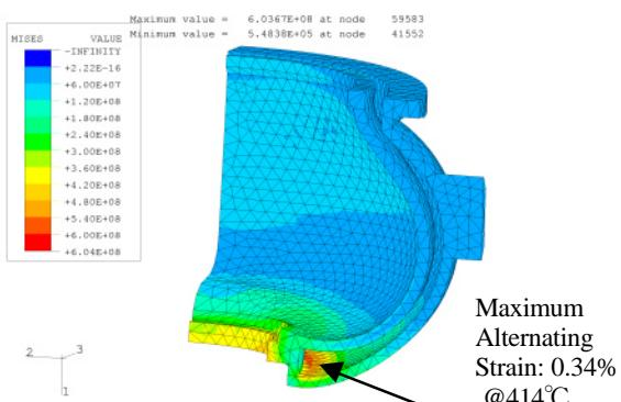
**Fig.8 A FEM analysis example of the RGT3R Turbine Casing (SCH11)**
