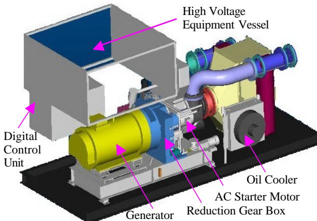
**Fig.14 The Latest equipment's configuration in the Gene-set Enclosure**
