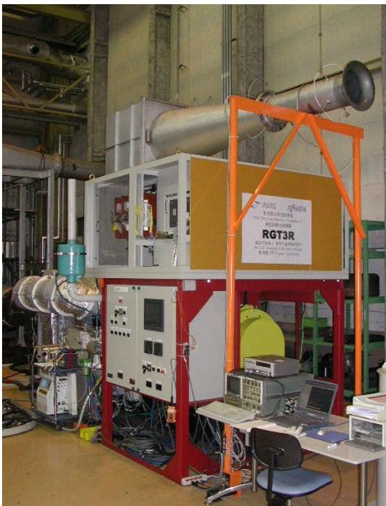
**Fig.18 Prototype of RGT3R Engine Test Rig (Completed)**
