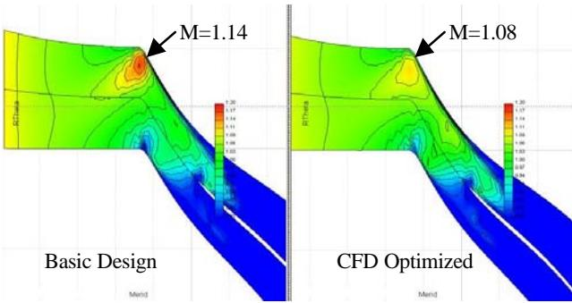
**Fig. 3 Relative Mach Number distribution at the impeller inducer tip area.**
