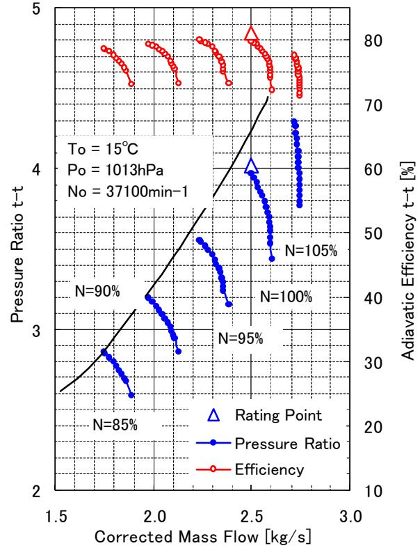
**Fig. 5 Test Results of CFD Optimized Compressor Performance**
