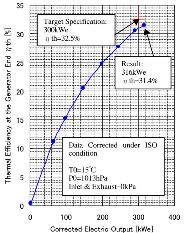
**Fig.19. Thermal Efficiency of prototype RGT3R**
