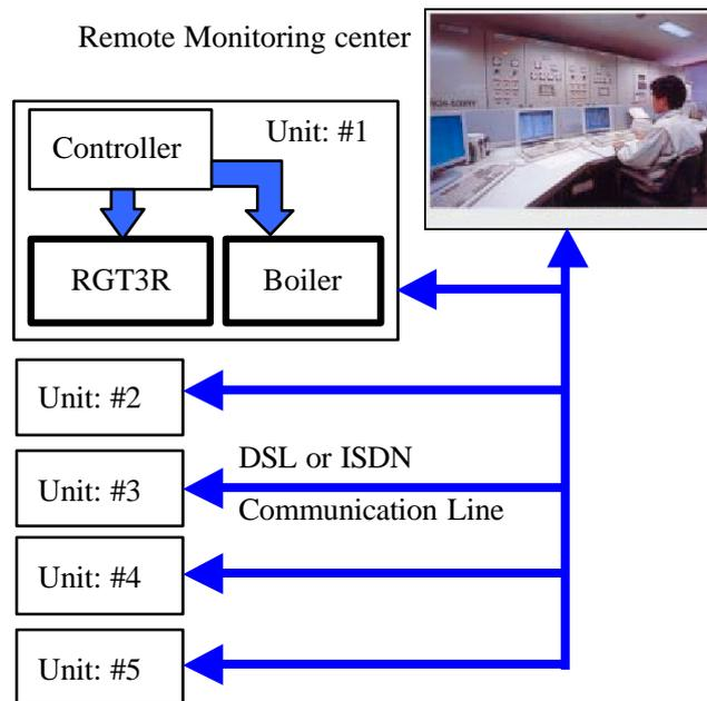
Fig.16 A Schematic of Remote Monitoring System
