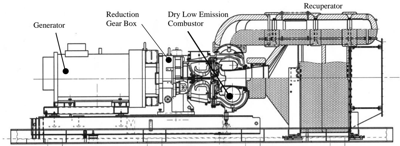
**Fig. 2 Cross Sectional View of RGT3R**
