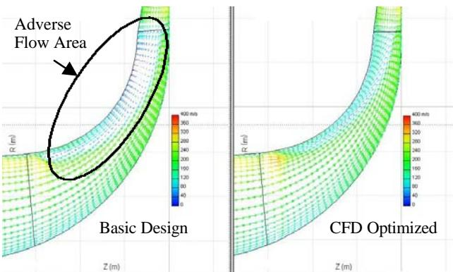
**Fig. 4 Relative velocity vector distribution comparison at the suction side of the impeller splitter blade.**
