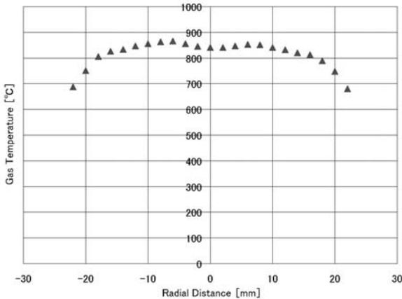
Fig. 5 Temperature uniformity at the combustor outlet atmospheric pressure, mean flow velocity = 12 m/s
