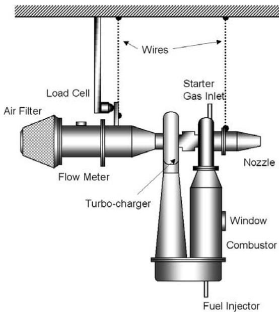
Fig. 2 Schematic of jet engine test system
