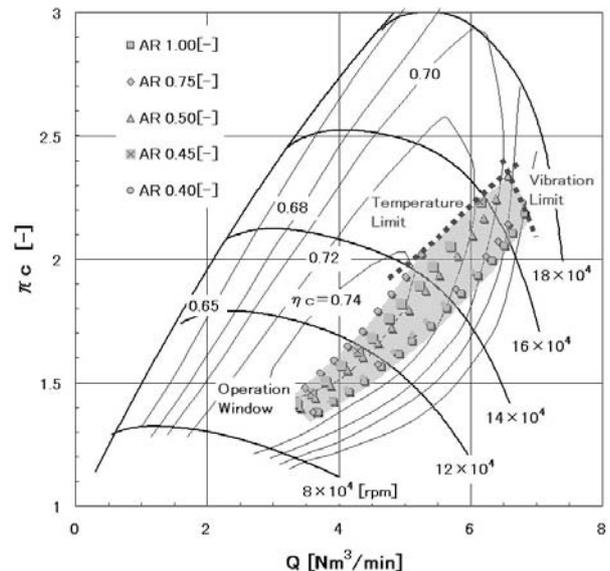
Fig. 7 Compressor operation window
