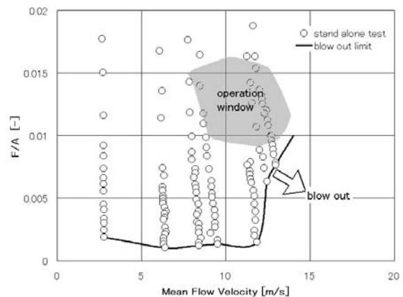
Fig. 4 Blow-out limit of the combustor
