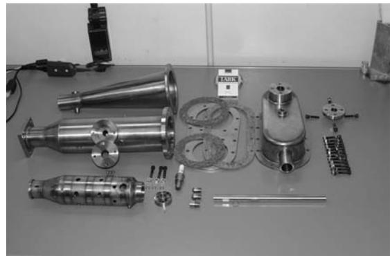
Fig. 3 Combustor Elements (disassembled)
