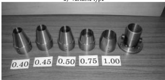
b) replaceable type (area ratio is noted)
