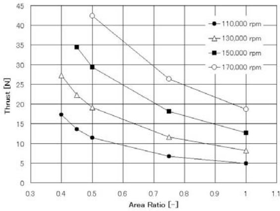
Fig. 8 Thrust dependence on nozzle area ratio
