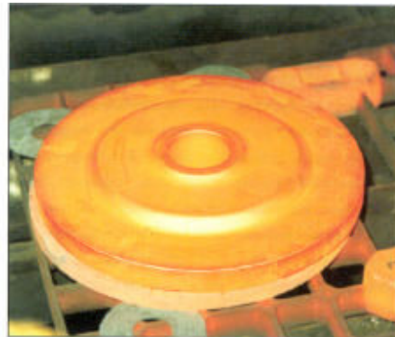
Figure 9. Boeing 737-size disk forging from new alloy.
