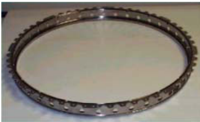
Fig. 19 TiAl shroud support for HTCE test
