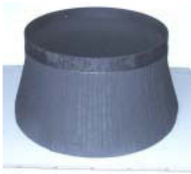
Fig. 14 CMC Combustor Inner Liner
