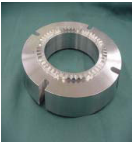
Fig.16 TMC Fan rotor sub-scale model ring for spin test
