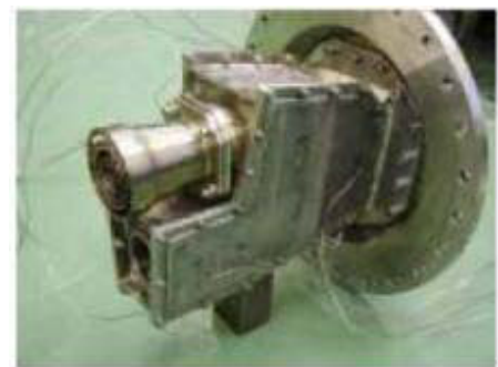
Fig. 4 Single sector of LPP combustor (1/16 model)
