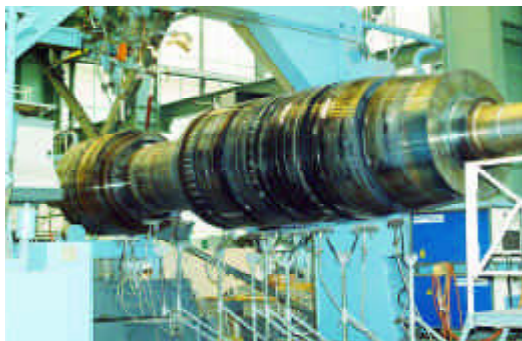
Fig 6: Manufacture of a welded rotor in Birr, Switzerland
