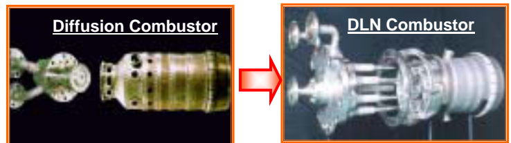
Fig. 9 Modification for DLN combustion system
