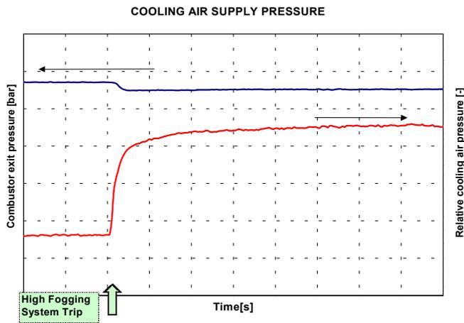
Figure 6 Relative pressure of the medium pressure cooling air system, and inlet pressure of the low-pressure turbine during a trip of the High Fogging system
