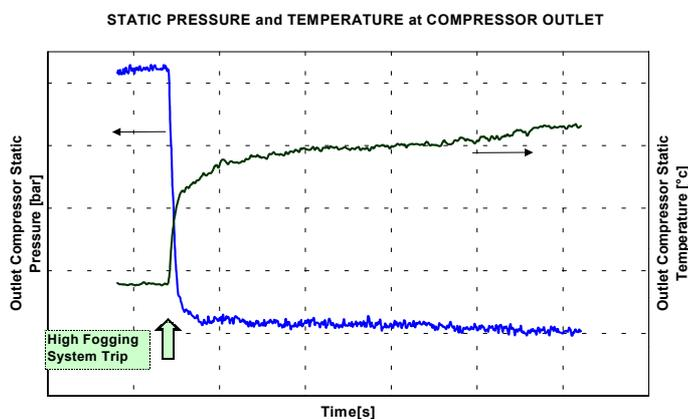
Figure 7 Relative high pressure cooling air supply pressure and temperature during a trip of High Fogging system
