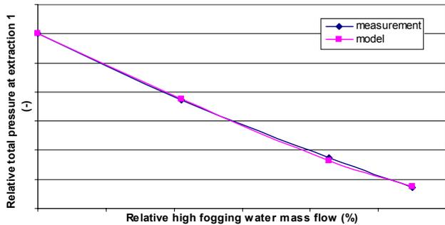
Figure 12 Compressor extraction 1 relative total pressure
