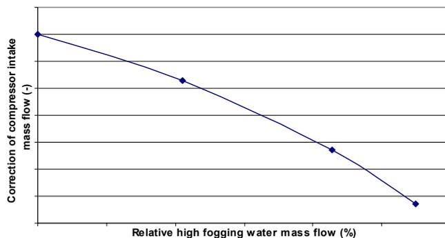
Figure 10 Compressor intake mass flow correction relative to the dry compressor
