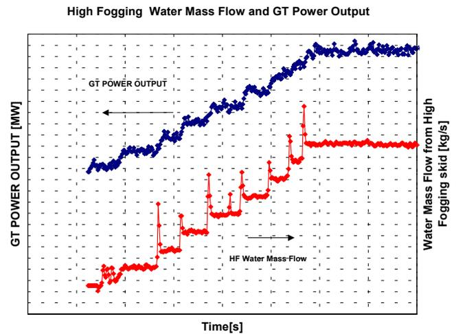
Figure 3 Power of the GT26 with High Fogging over time with stepwise increase of the High Fogging water mass flow (peaks in water mass flow are measurement errors during fast transient).
