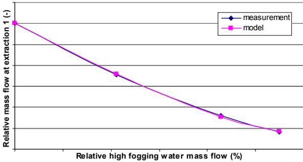
Figure 11 Compressor extraction 1 relative mass flow
