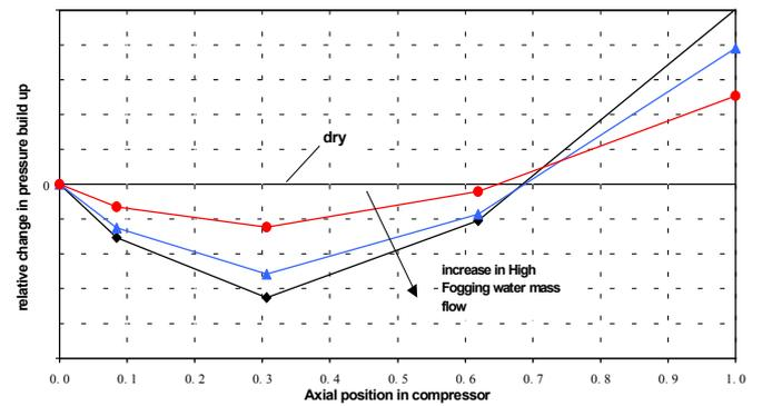
Figure 5 Typical change in compressor pressure build up due to High Fogging relative to dry operation
