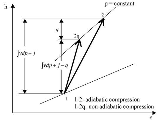
Figure 8 h-s diagram showing both adiabatic and non-adiabatic compression processes
