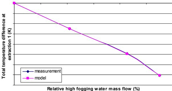
Figure 13 Compressor extraction 1 total temperature difference
