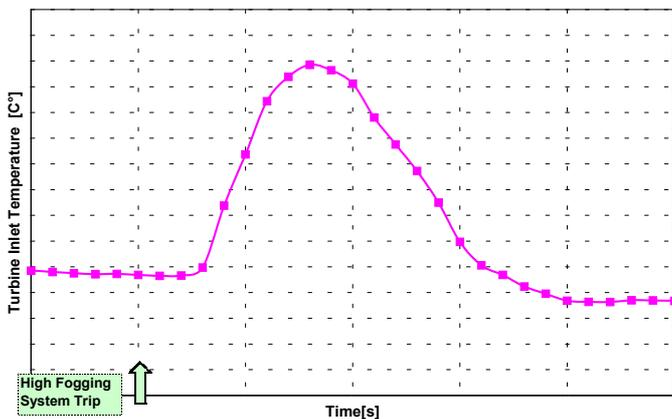
Figure 4 Transient changes of the turbine inlet temperature with High Fogging with conventional control logic.
