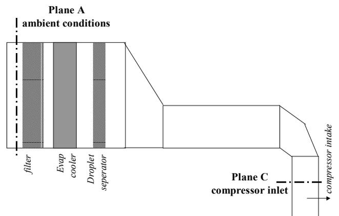
Figure 1 Schematic overview of an air intake with an evaporative cooling system.
