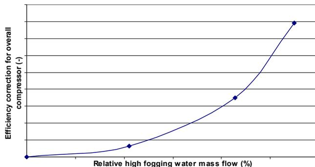
Figure 9 Efficiency correction factor for overall compressor relative to the dry compressor
