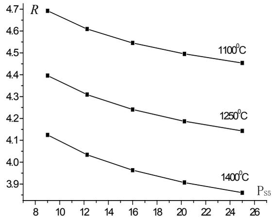
Fig.5 The mass flow ratio of the cycle
