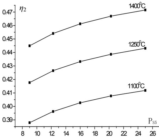
Fig.4 Exergy efficiency for different cycle maximum pressure and temperature
