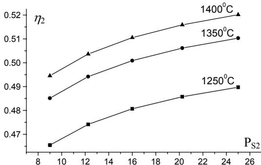
Fig.7 Exergy efficiency of modified cycle
