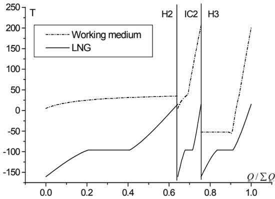
Fig.3 T-Q diagram of LNG vaporizing processes
