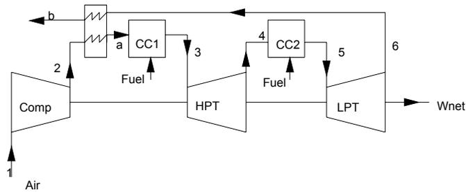
**Figure 2: Flow diagram of reheat heat exchanger cycle (RHC)**
