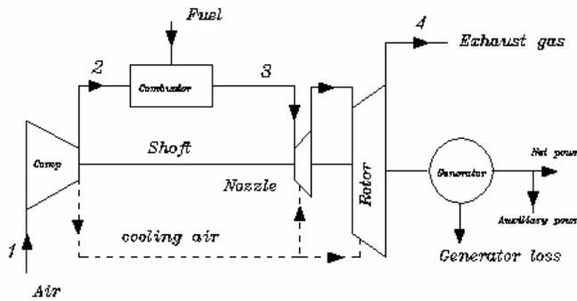
**Figure 3: Flow diagram for cooled turbine model**
