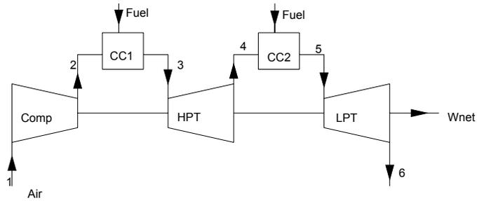
**Figure 1: Flow diagram of reheat cycle (RC)**
