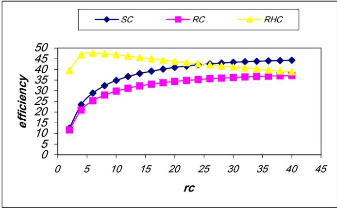
Figure 6: Efficiency versus pressure ratio using uncooled turbine model
