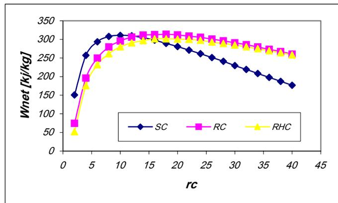
Figure 9: Specific net work versus pressure ratio using cooled turbine model
