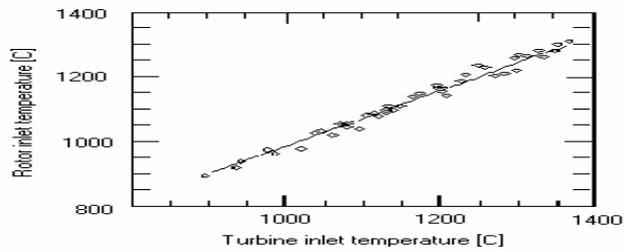
**Figure 4: Rotor inlet temperature against turbine inlet temperature for various gas turbines**
