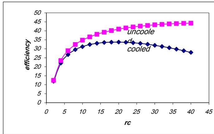
Figure 8: Comparison of variation of SC efficiency against pressure ratio using both cooled and uncooled turbine models
