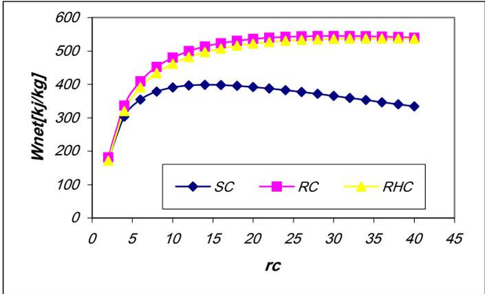
Figure 5: Specific net work versus pressure ratio using uncooled turbine model
