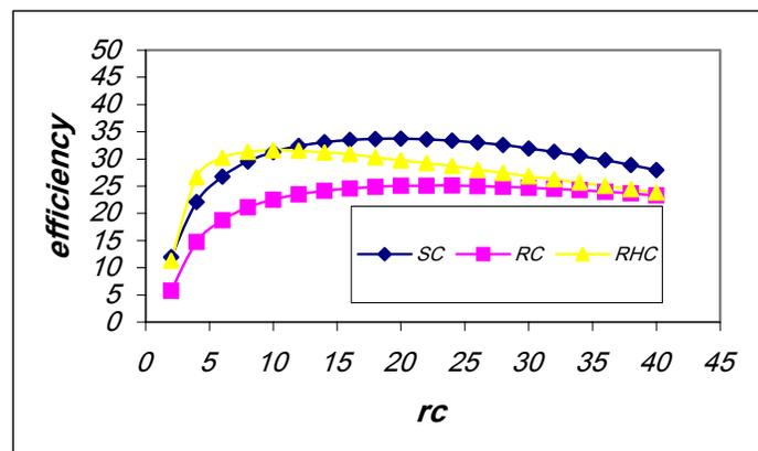
Figure 10: Efficiency versus pressure ratio using cooled turbine model
