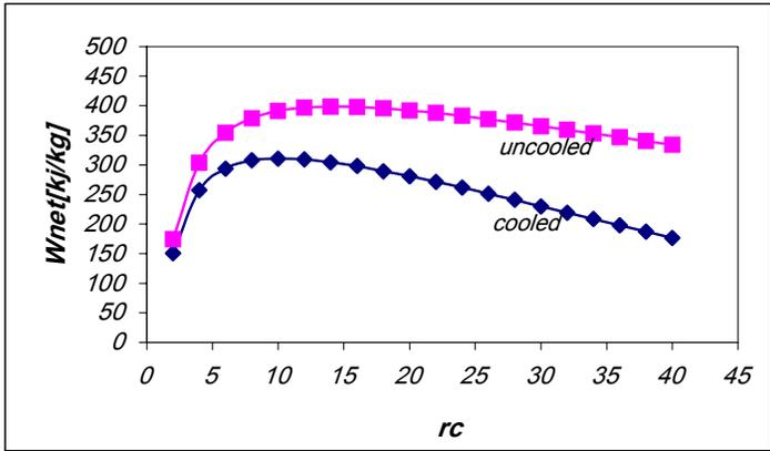
Figure 7: Comparison of variation of SC specific net work against pressure ratio using both cooled and uncooled turbine models
