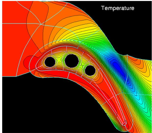
Fig.5: Result with Emulation of Coolant
