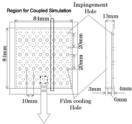
Fig.10: Configuration of Basic and Fine Specimen
