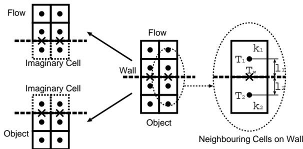
Fig.2: Connecting Boundary of Flow and Object
