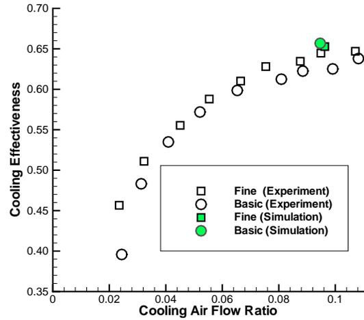
Fig.14: Comparison of Cooling Effectiveness at Gas Speed of  $Re = 7.0 \times 10^5$
