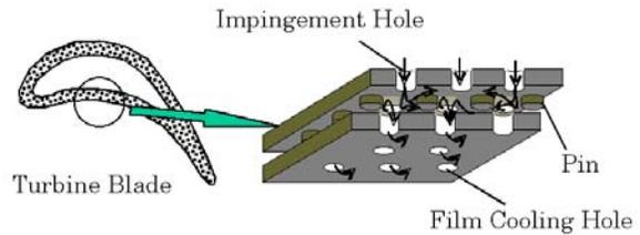
Fig.9: Concept of Integrated Cooling Configuration
