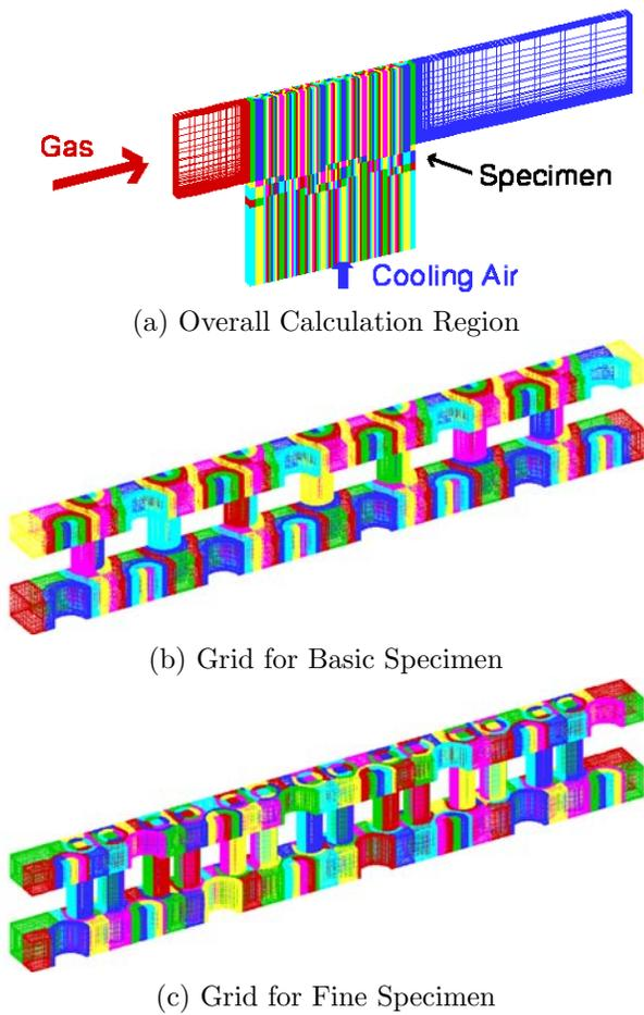
Fig.13: Numerical Grid for Basic and Fine Specimen
