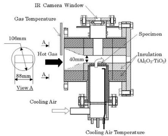
Fig.11: Test Section Detail
