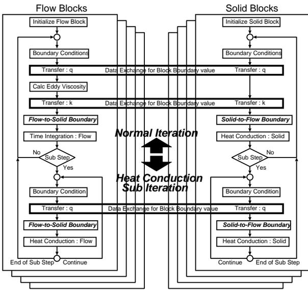
Fig.6: Program Flow with Sub-iteration
