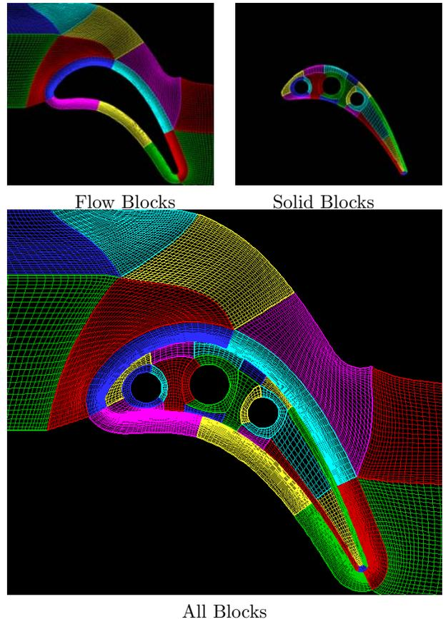
Fig.3: Numerical Grid of 2D Turbine
