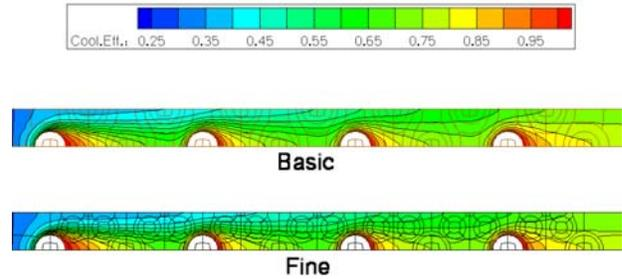
Fig.15: Cooling Effectiveness Distribution on Specimen Surface
