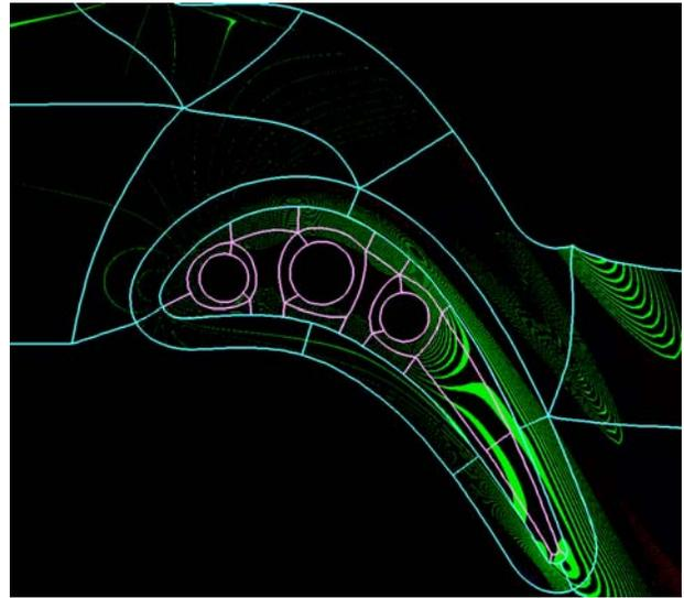
Fig.8: Difference of Temperature with/without Sub-iteration
