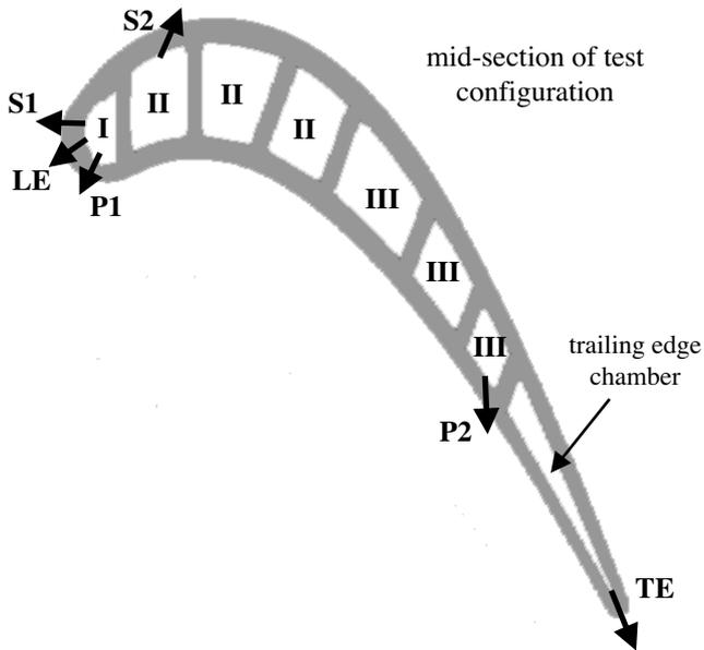
Fig. 1 Film-cooled test blade
