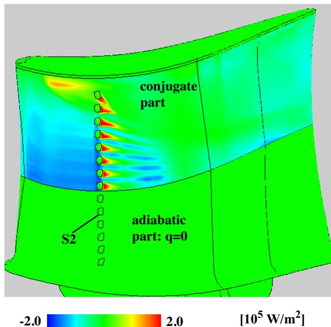
Fig. 10 Specific heat transfer distribution on the suction side
