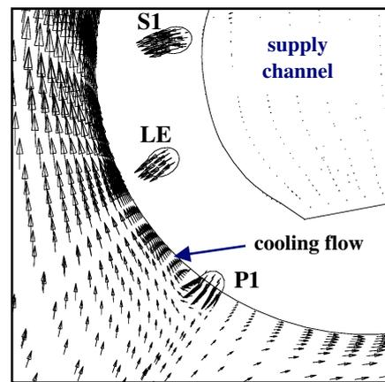
Fig. 4 Zoomed view of leading edge (radial cutting plane in mid-section), flow vectors
