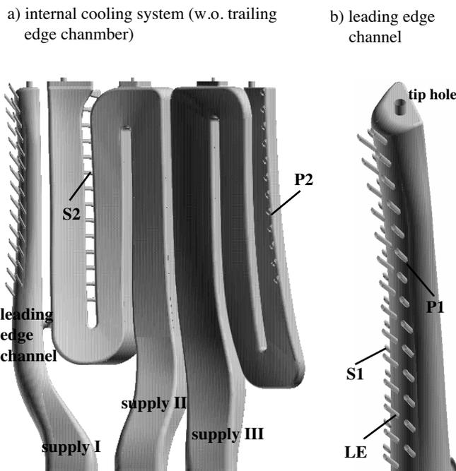
Fig. 2 Internal cooling system of test configuration
