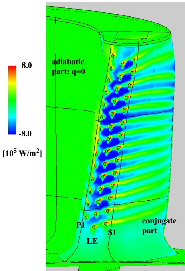
Fig. 7 Specific heat transfer distribution at the leading edge
