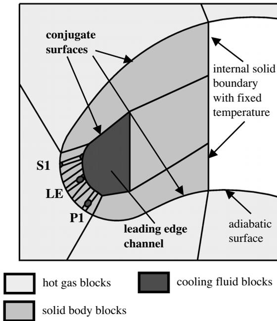
Fig. 3 Illustration of the blade leading edge model for the CCT
