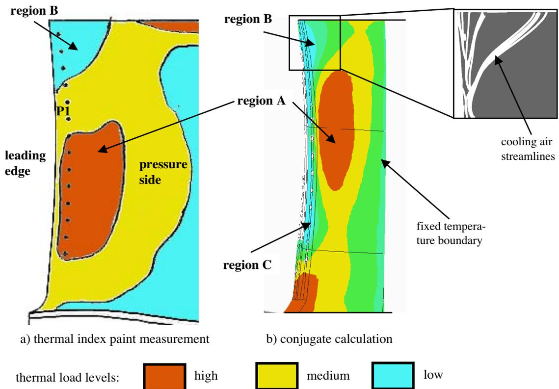
Fig. 6 Comparison of thermal index paint experiment and conjugate calculation of the leading edge region (pressure side)
