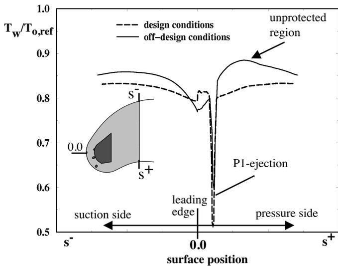
Fig. 5 Surface temperature distribution in leading edge area
