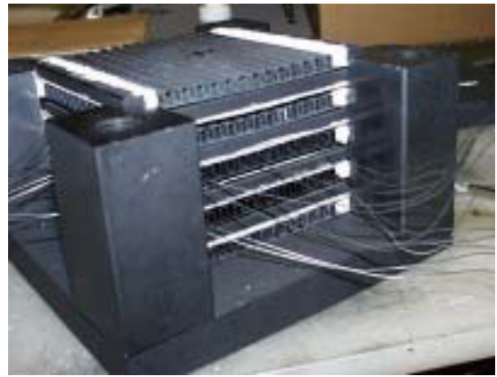
Fig.2 General view of the heat transfer test model under its assembly
