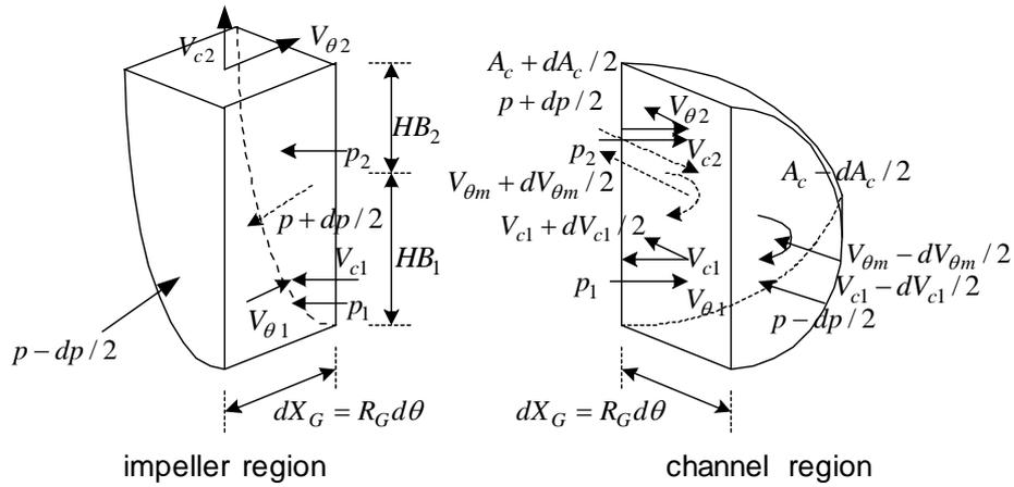
Figure (4). Control volumes representing section  $d\theta$  of open channel and impeller
