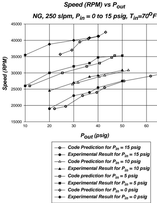
Figure (12) Theoretical and test data overlapped for flow rate 250 slpm
