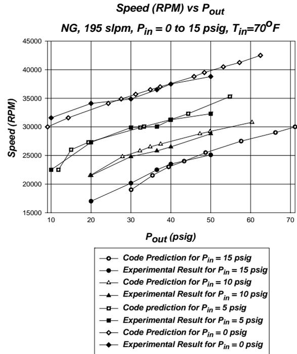
Figure (11) Theoretical and test data overlapped for flow rate 195 slpm
