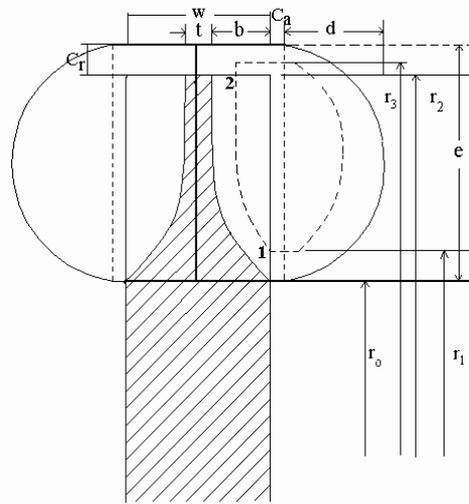
Figure (5). Schematic of blade and channel geometry
