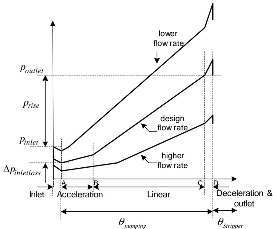
Figure (3) Tangential pressure variation in a regenerative turbomachine
