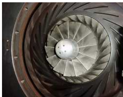
Figure 2. Photo of the open stage with backswept rotor and vaned diffuser.
