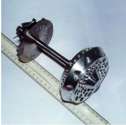
Fig. 7 GTE rotor of 60 KW power (centrifugal compressor and tunnel turbine) after assembly and balancing.
