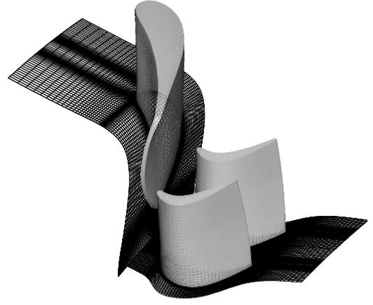
Fig. 12 CFD grids of 1<sup>st</sup> stage of commercial gas-turbine
