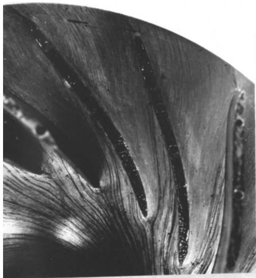
Fig. 18 Flow traces at the hub surface of the impeller 085/065, \Phi_{des} = 0.085 . “Water” test rig visualization (Gerasimov, 1982)
