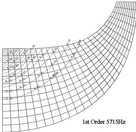
Figure 2 Resonance Frequency Analysis for the Compressor Blade TYPE-C1
