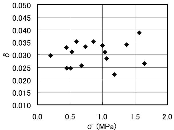
Figure 9 Logarithmic Decrement by Hammering Test
