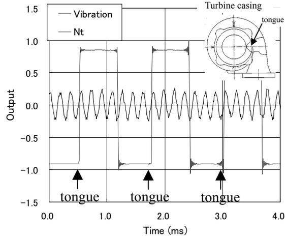
Figure 5 Rotational Speed and Blade Vibration by 7th Engine Order Excitation Force
