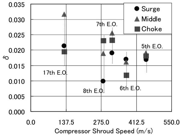
Figure 10 Logarithmic Decrement of the Compressor Blade TYPE-C1
