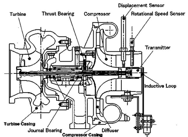
Figure 1 Cross-Section of Test Machine
