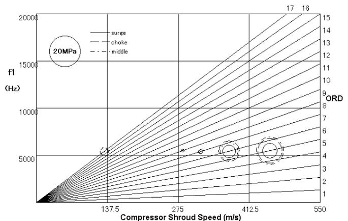
Figure 4 Campbell Diagram of the Compressor Blade TYPE-C1
