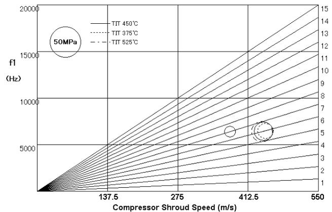
Figure 6 Campbell Diagram of the Turbine Blade TYPE-T1
