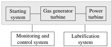
Fig. 1 Gas turbine main components (OREDA, 1999)
