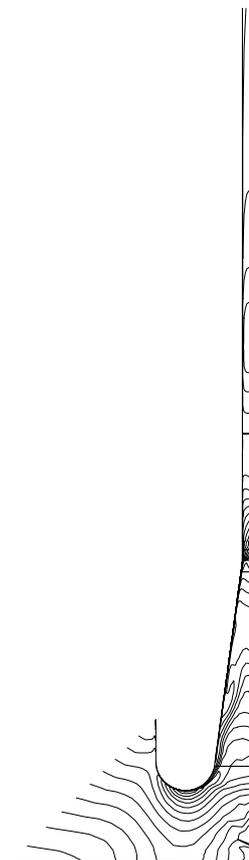
Fig.3. Mach number contours in mean meridional section.
