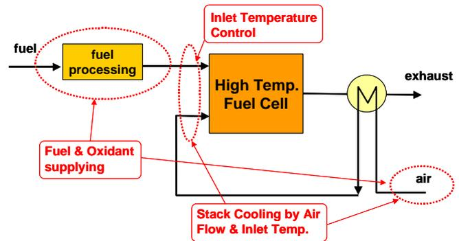
Figure 2 Basic configuration of HTFC system
