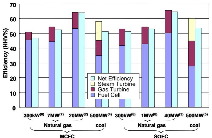
Figure 4 Typical system efficiency of various HTFC combined systems<sup>(2)-(9)</sup>
