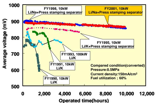
Figure 5 Average cell voltage history of the short stack comparing former tested stacks
