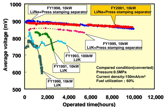
Figure 5 Average cell voltage history of the short stack comparing former tested stacks
