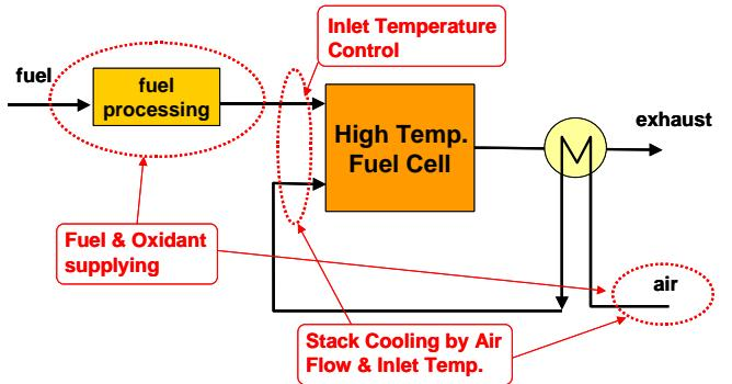
Figure 2 Basic configuration of HTFC system
