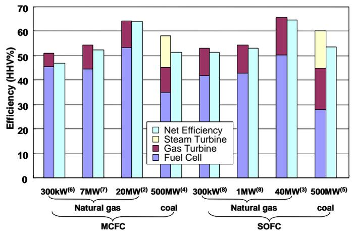
Figure 4 Typical system efficiency of various HTFC combined systems<sup>(2)-(9)</sup>
