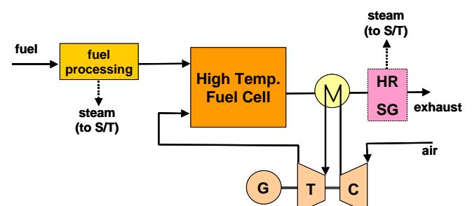
(b) HTFC atmospheric operation
