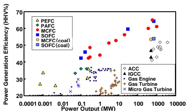
Figure 1 Power generation efficiency with output capacity in various systems
