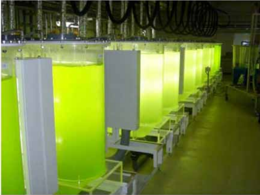
Figure 1. System for intensive high density culture of phytoplankton.
