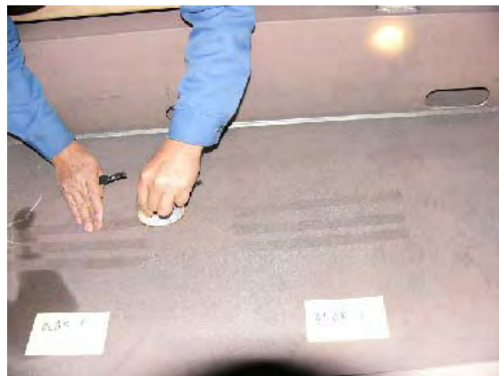
Photo.2 Dust measurement on the floor surface
