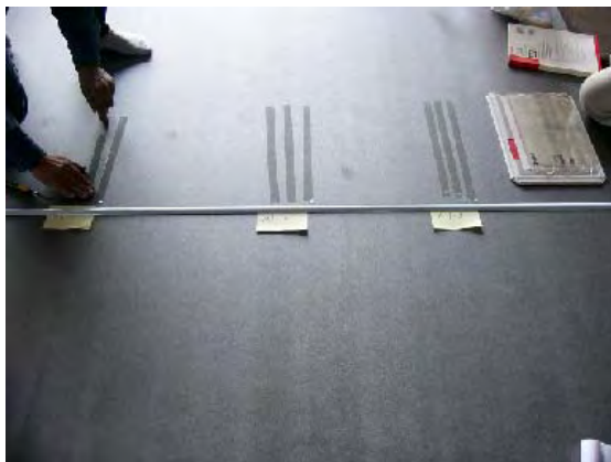
Photo.3 Dust measurement on the shot blasted steel plate
