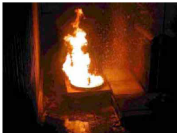
42 s after ignition (Start of form discharge)
