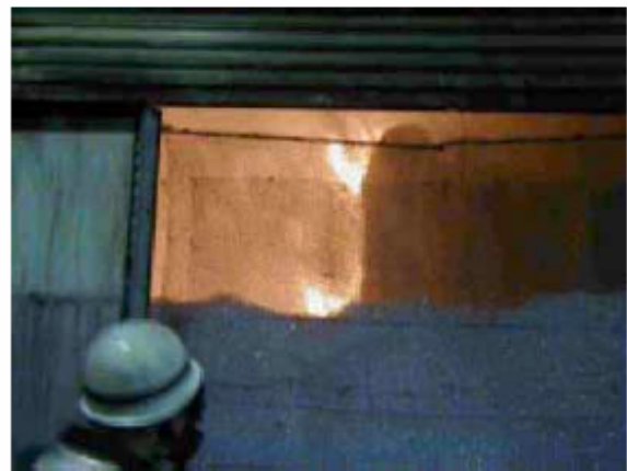
232s after ignition (220s after form discharge) Height of form discharged: 2m
