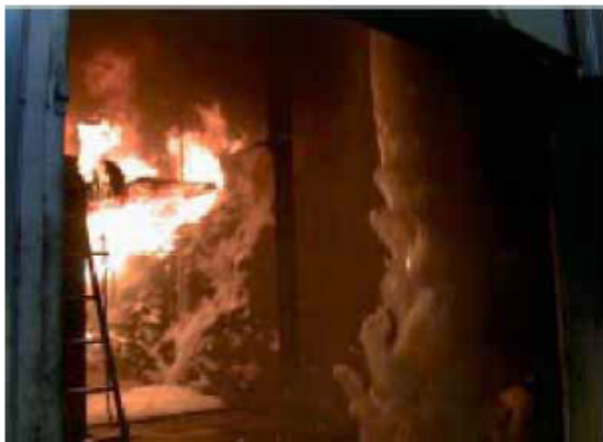
Start the Foam discharge after 12 seconds pre-burn.
