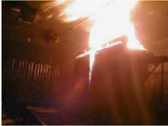
3m 2 Tray fire on the test mock-up Started flowing heptane fire.
