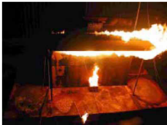
Low-pressure low flow concealed horizontal spray fire (1 MW fire) and 0.1m 2 pool fire
