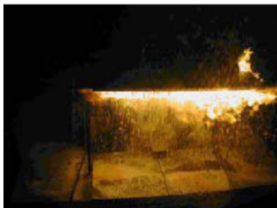
149 s after ignition (12 s after system activated). Extinguished 0.1m 2 pool fire 1 MW spray fire still remaining.
