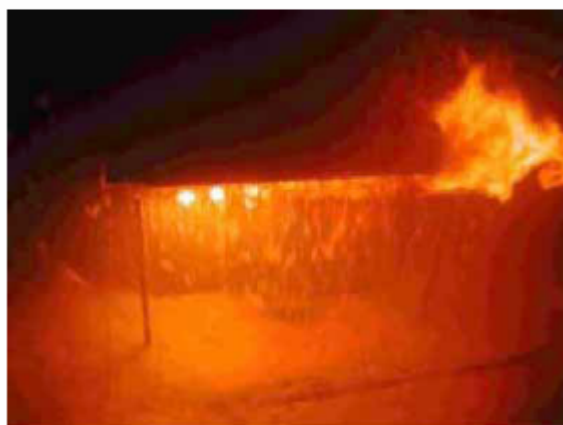
205 s after ignition (68 s after system activated). Floor was covered by form discharged.
