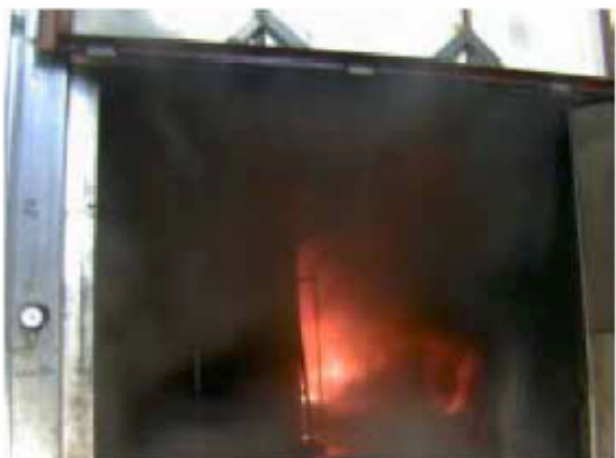
30 seconds after Foam discharge. The foam attacks the tray fire.
