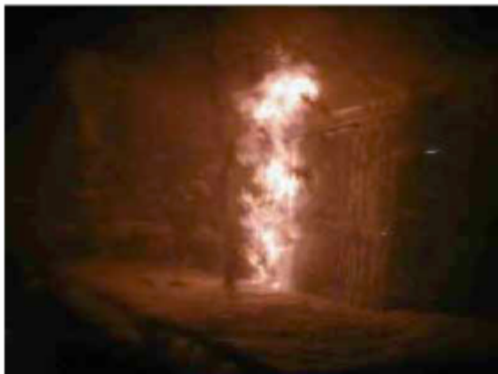
62s after ignition (50s after form discharge) 3m 2 Tray fire and flowing heptane fire are still burning
