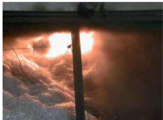
130 seconds after Foam discharge. The foam attacks the spray fire.
