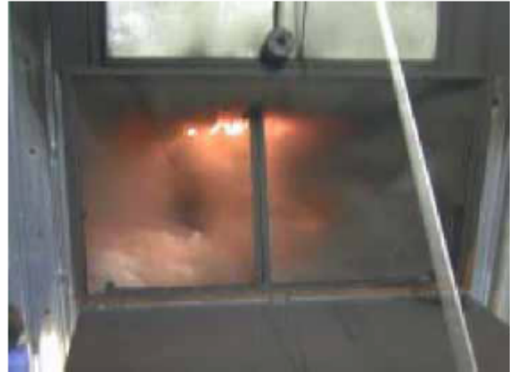
100 seconds after Foam discharge. The foam attacks the spray fire.
