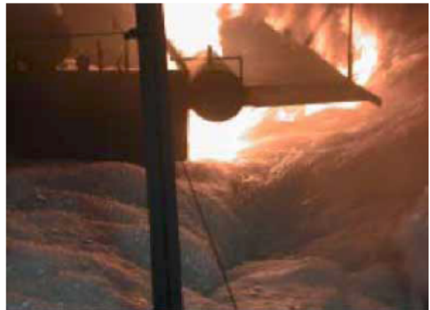
65 seconds after Foam discharge. The foam attacks the spray fire.
