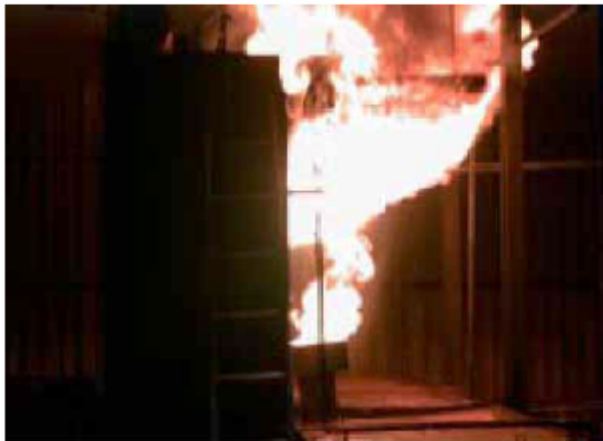
Start the Diesel Oil spray fire.
