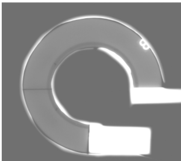
Fig.15 Over all picture of X-ray radiography of the TMC ring after over speed test
