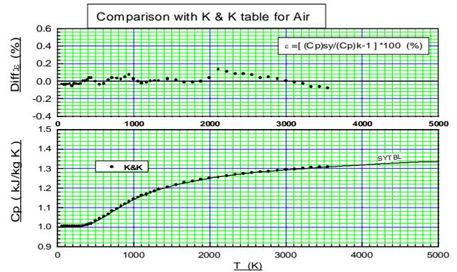
Fig. 3 Cp compared with Keenan's table for air
