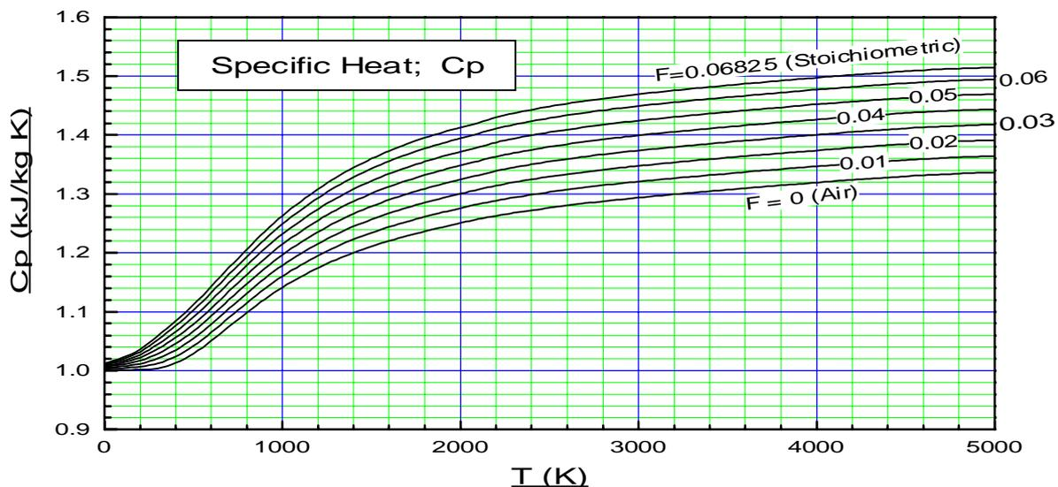
Fig.1 Specific heat characteristics
