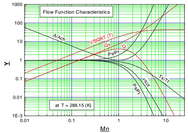
Fig. 8 Flow function characteristics
