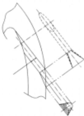
Figure 9 Shaped film cooling hole configuration
