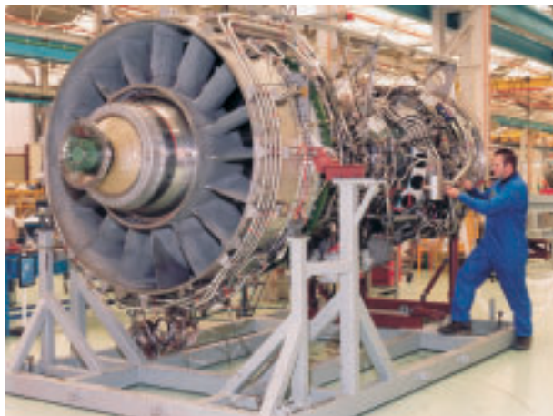
Fig 5 MT30 following build
