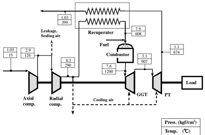
Fig.4 The Engine Cycle
