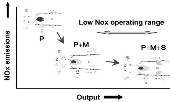
Fig.9 Burning Control Method
