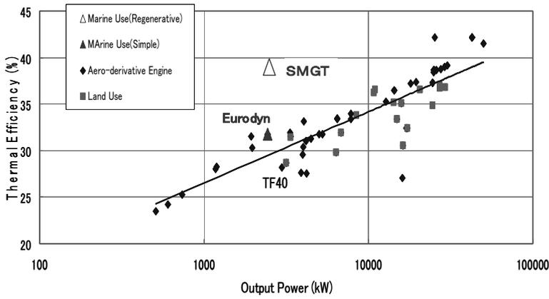
Fig.1 Thermal Efficiencies of Marine Gas Turbines
