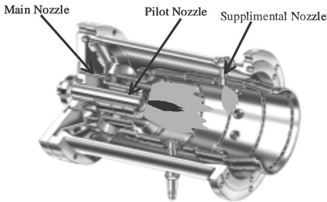
Fig.8 Cross-sectional View
