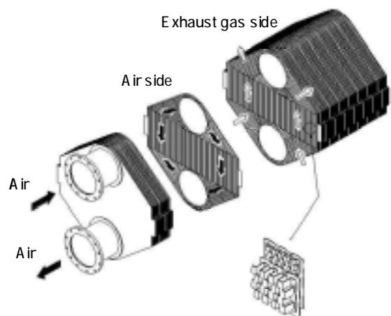
Fig.12 Configuration of Core for Plate-fin Recuperator
