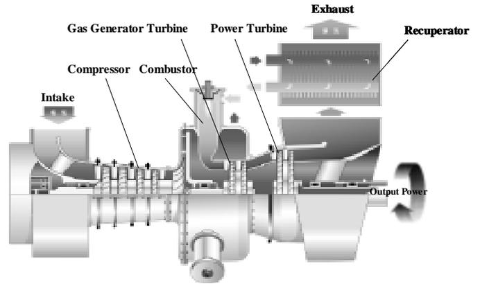
Fig.3 Cross Sectional View of SMGT
