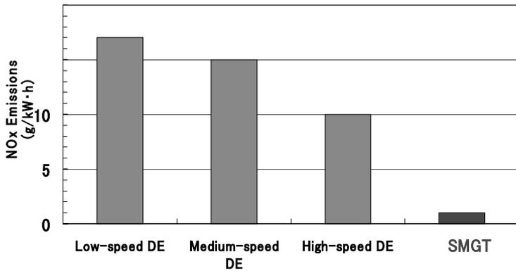
Fig.2 Comparison of NOx Emissions with Diesel Engines
