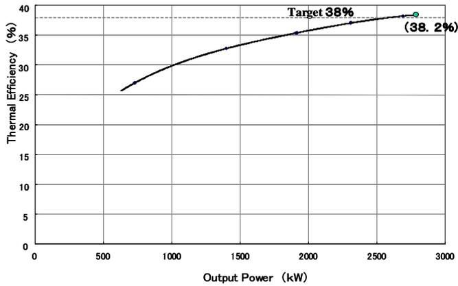
Fig. 16 Results of Thermal Efficiency
