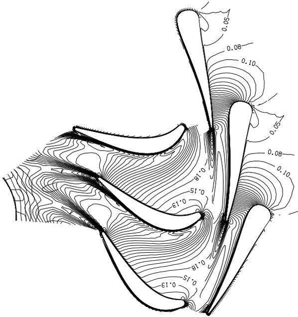
Fig.4. Mach number contours at mean section of flow passage (Version: Nozzle1+Rotor1).
