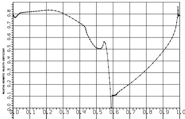
Fig.6. Isentropic Laval number distribution along the profile arc length of Rotor1 (mean section)
