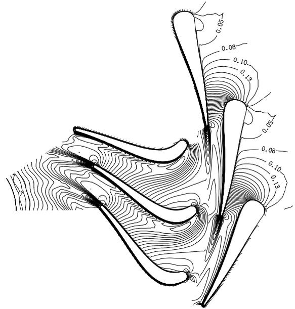
Fig.7. Mach number contours at mean section of flow passage (Version: Nozzle2+Rotor2).
