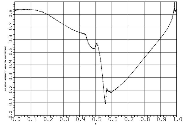
Fig.8. Isentropic Laval number distribution along the profile arc length of Rotor2 (mean section)
