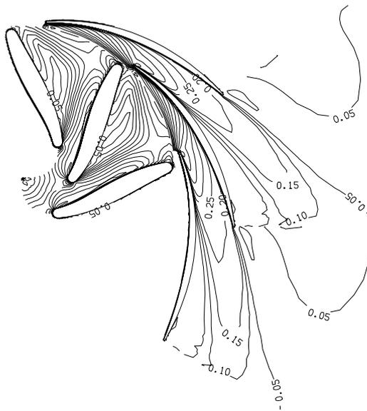
Fig.1. Mach number contours close to hub section.
