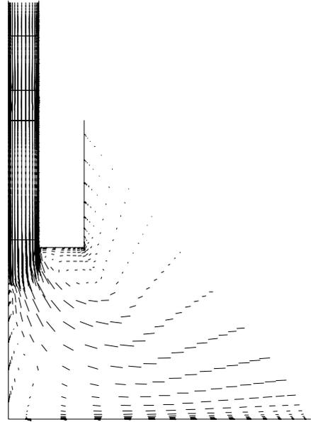
Fig.10. Velocity vector field in mean blade-to-blade section.
