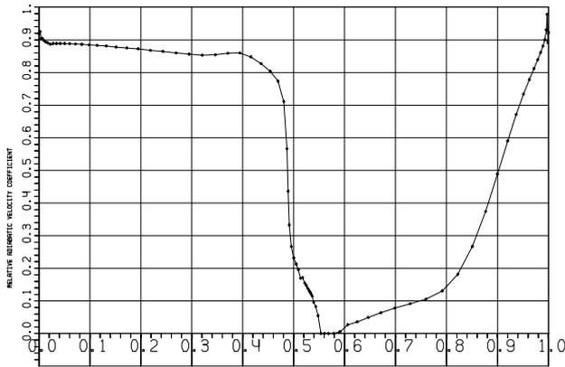
Fig.5. Isentropic Laval number distribution along the profile arc length of Nozzle1 (mean section)
