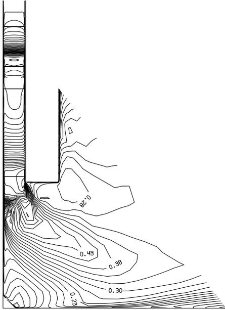
Fig.9. Mach number contours in mean blade-to-blade section.
