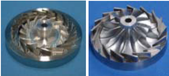
Fig.11 2D and 3D radial turbines for perm top gas turbines (14)
