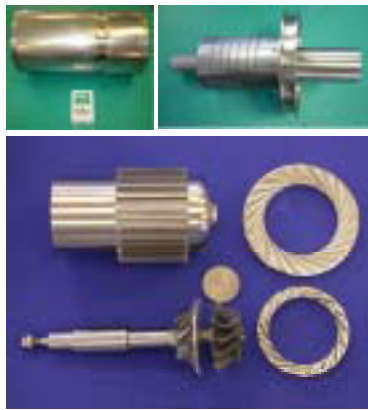
Fig.7 A palm top gas turbine and its parts
