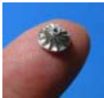
Fig. 8 A turbine wheel of a finger top GT Diameter 8mm
